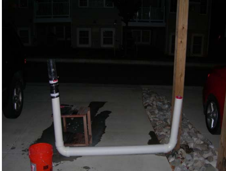
Figure 4.7: Assembled Falling Head Permeability Test
