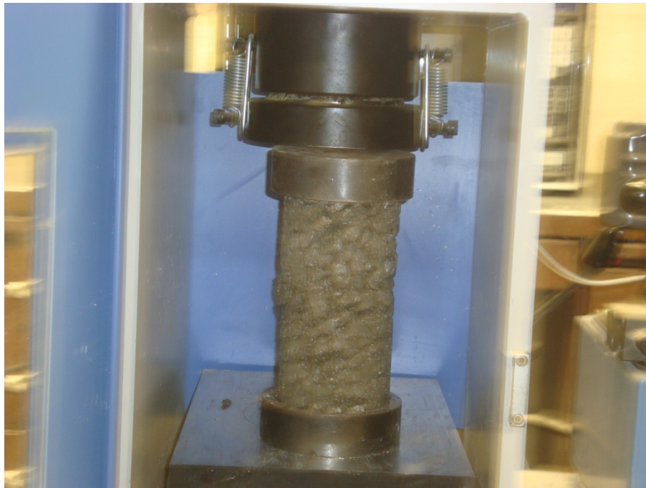
Figure 4.2: Pervious Concrete Specimen in Compression Testing Machine
