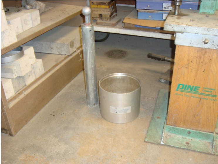
Figure 4.1: Apparatus Used for Density and Void Content
