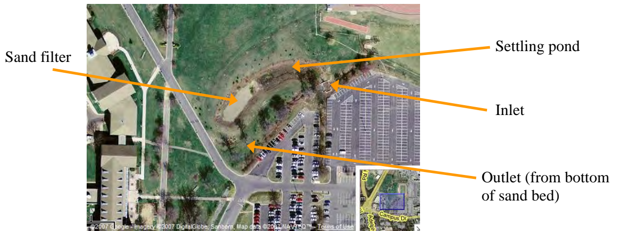
Figure 1. Aerial view of UMUC sand filter site
