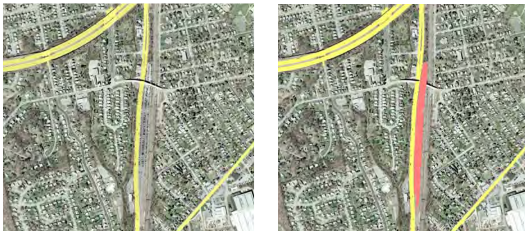
Figure 1-8 CADD Drawing Converted and Clipped into GIS Impervious Layer
