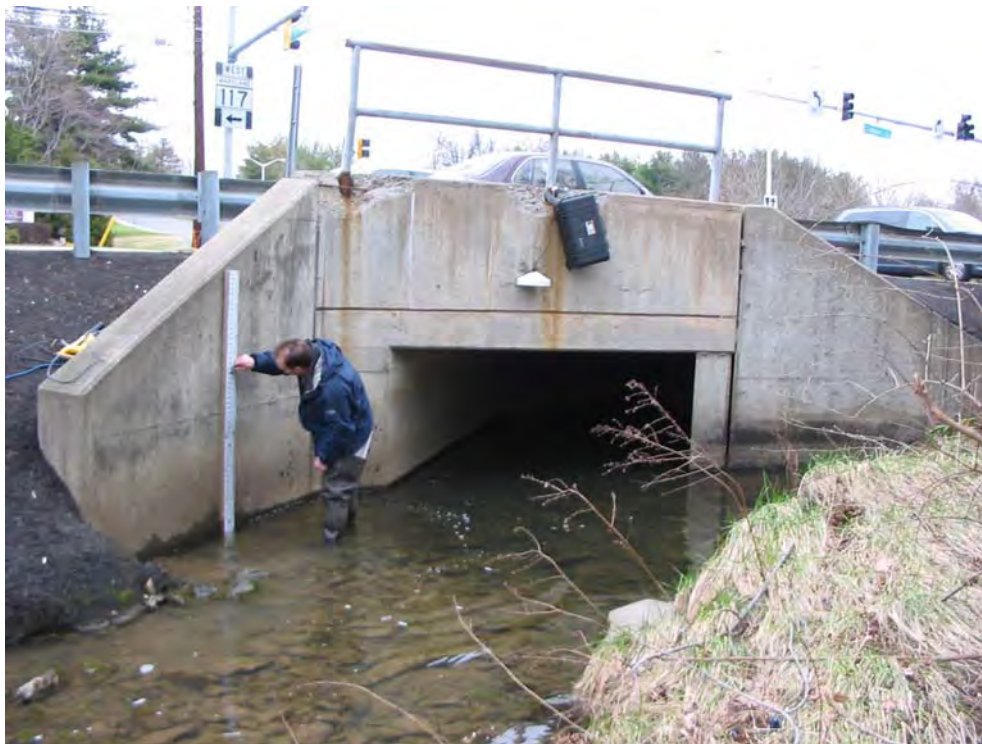
Figure 2.2: Continuous water level meter at upstream monitoring site
