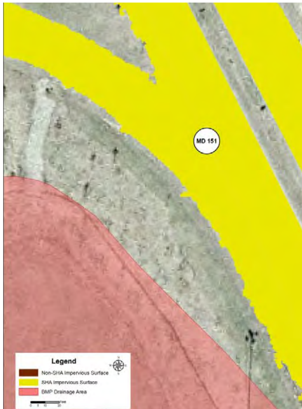
Figure 1-5 Impervious Surface Layer Generated with Feature Analyst Process
