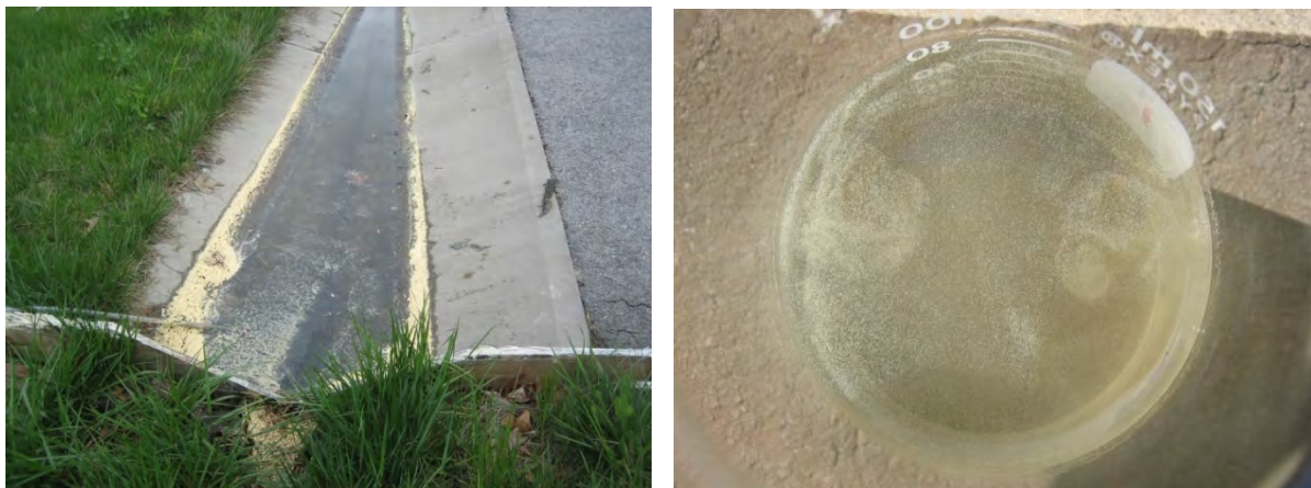
Figure 1. Pollens from storm water runoff on April 29 th ; (a) Pollen in direct channel, and (b) Pollens in the first flush sample.
