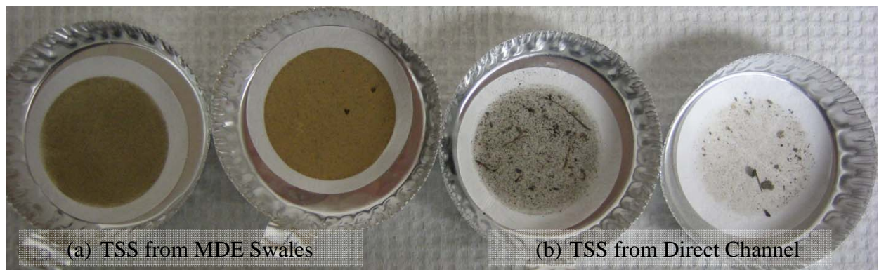
Figure 3. Captured suspended solids on grass fiber filter (a) from MDE swales, and (b) from direct channel.
