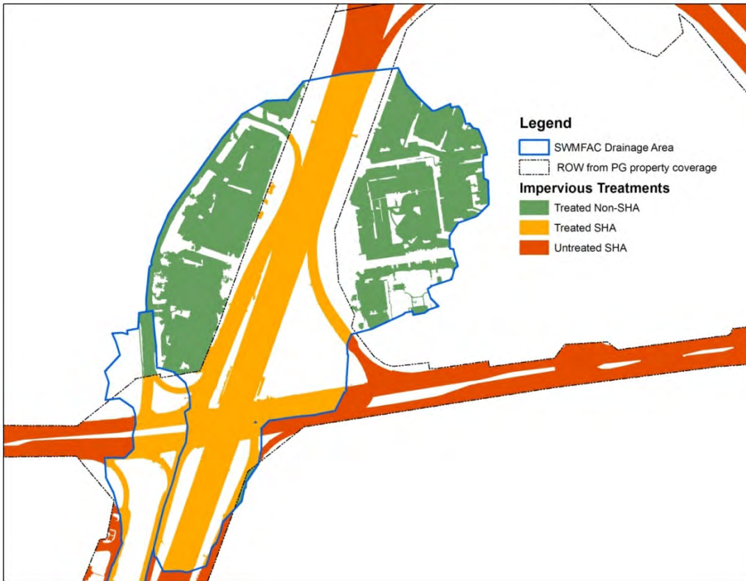
Figure 1-3 Example of Impervious Layer
