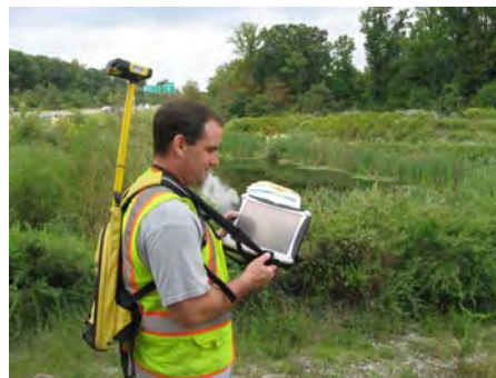
Figure 3-14 GPS and Field Tool Used for Efficient Data Entry During BMP Inspections
