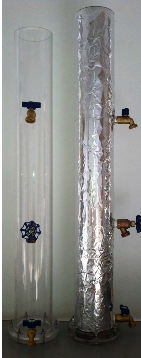
Figure 5: Constructed model bioretention system columns
