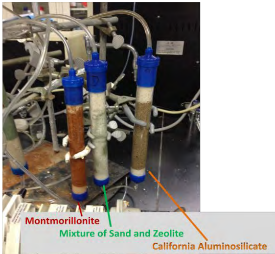
Figure 1-8 Modified Conventional Sand Filter Testing
