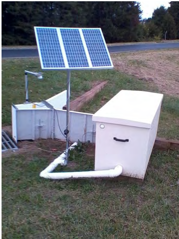
Figure 1-40: Bioswale Monitoring Equipment
