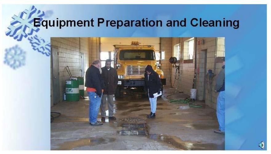
Clean equipment in wash bay so that wash water is treated by the grit separator and oil/water separator to minimize the discharge of sediment, salt and heavy metals into the environment.
