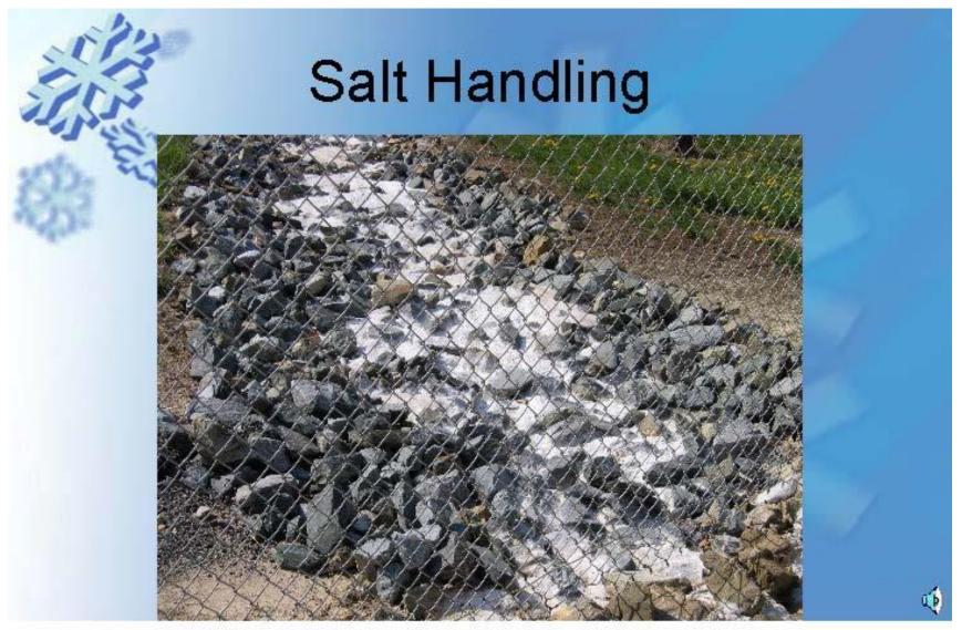
Impact of a salt/abrasive mix not being placed under cover. Non-compliant with NPDES permit conditions.
