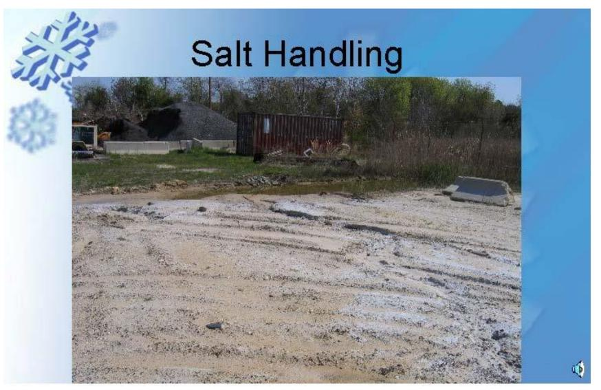
Mixing salt/abrasives on unpaved areas can result in destroying vegetation and causing an erosion problem.
