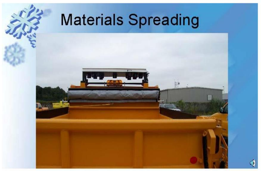
Keep your load covered. Use the tarp to reduce wind erosion of material
