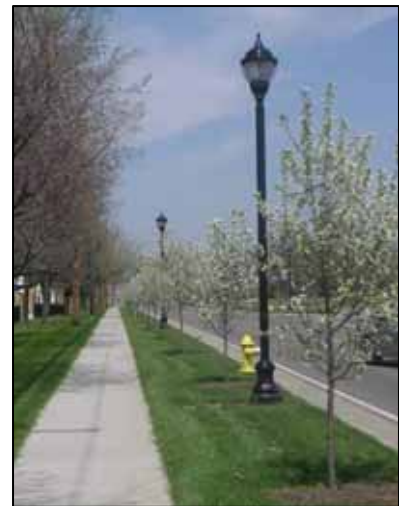
Figure 9.3 - Example: of a Sidewalk with Buffer Zone
