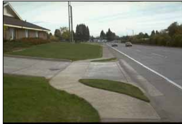
Figure 9.8 - Example of a Continuous Pedestrian Route over a Depressed Curb Entrance with Horizontal Deflection (An example application of Standard No. 630.01)
