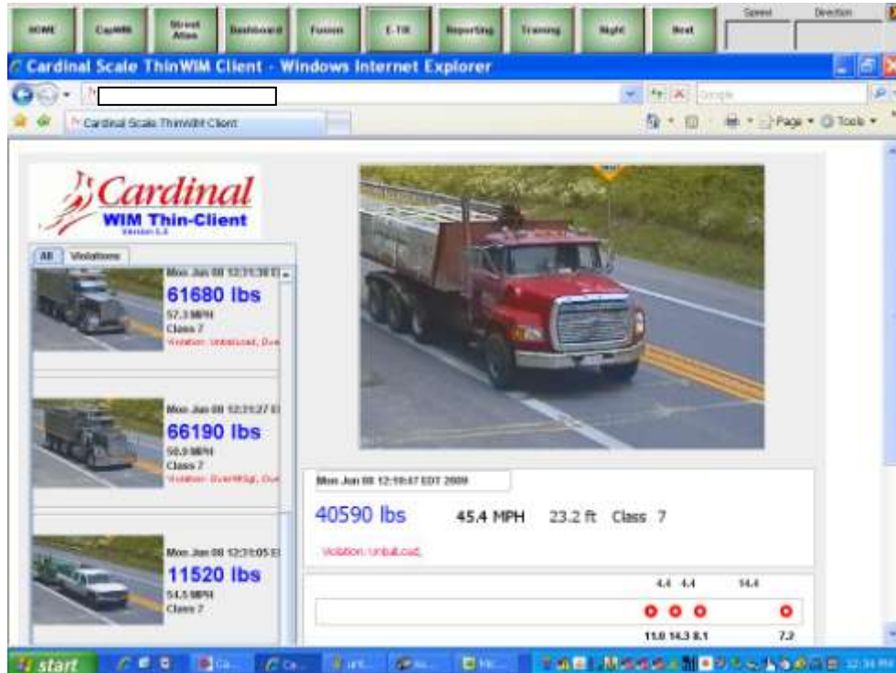
Figure 43. An Example of CMVs Screened by Unbalanced Load Indication
