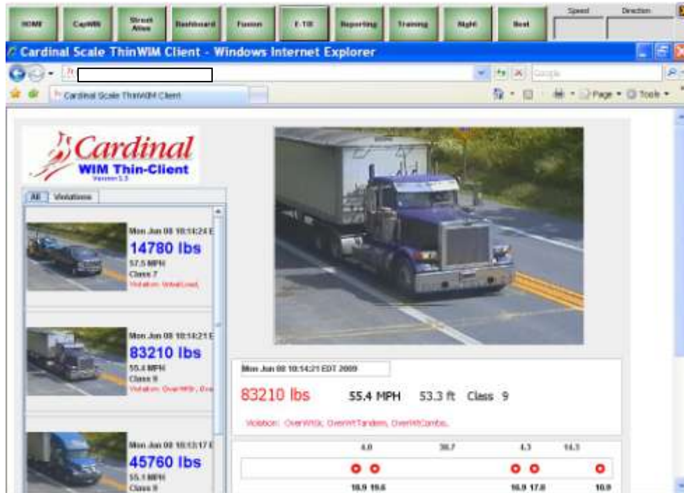
Figure 42. An Example of CMVs Screened by Over weight Indication
