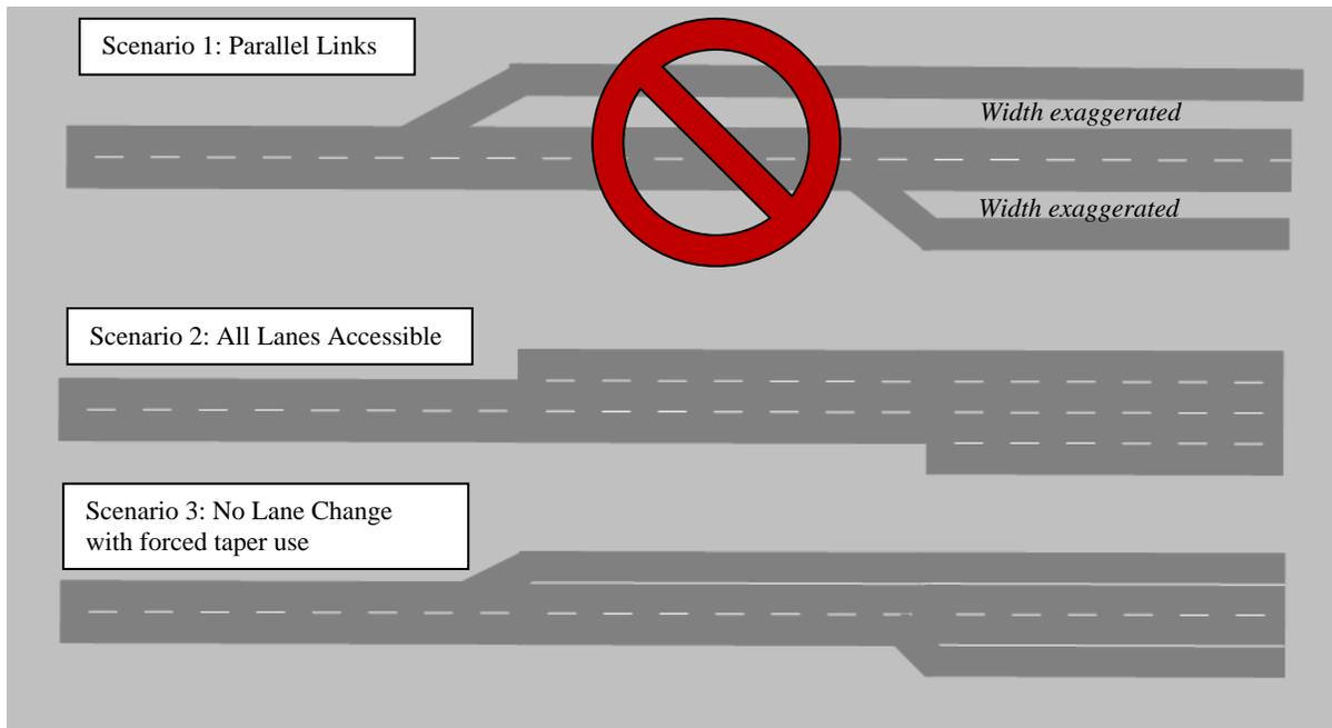
Merges and diverges with acceleration and deceleration lanes shall be modeled similarly (one link-all lanes), one link with the acceleration or deceleration lane included as part of the mainline link, as shown below, unless the existing conditions include a physical barrier between the mainline and the ramp lanes (ex. Collector-Distributor lane).
