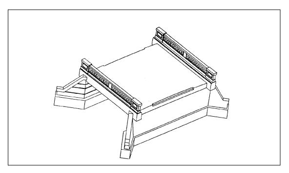
Figure 3.5. Isometric view of slab structure (Source: Maryland State Roads Commission, 1930 Standard Plans).
