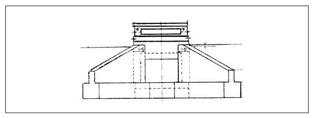
Figure 3.7. Box culvert from 1931 Standard Plans (Maryland State Roads Commission 1931). Note incised parapet.
