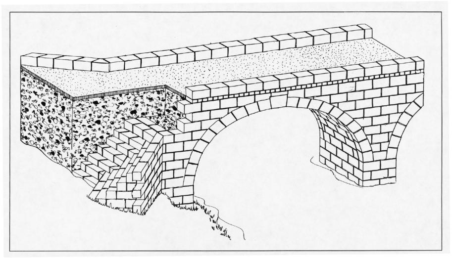
Figure 3.1. Isometric view of masonry arched structure (Source: Pennsylvania Historical and Museum Commission and Pennsylvania Department of Transportation 1986).
