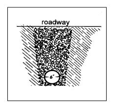
Figure 1.2. Drawing of a culvert (Adapted from Johnson 1899: 275)
