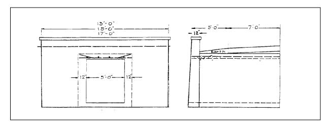
Figure 3.6. "Steel-concrete" box culvert, 1912 Standard Plans (Source: Maryland State Roads Commission 1912).
