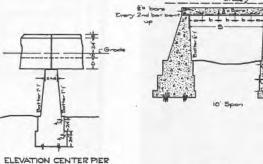
SECTION CENTER PIER DOUBLE SPAN SLAB BRIDGE
