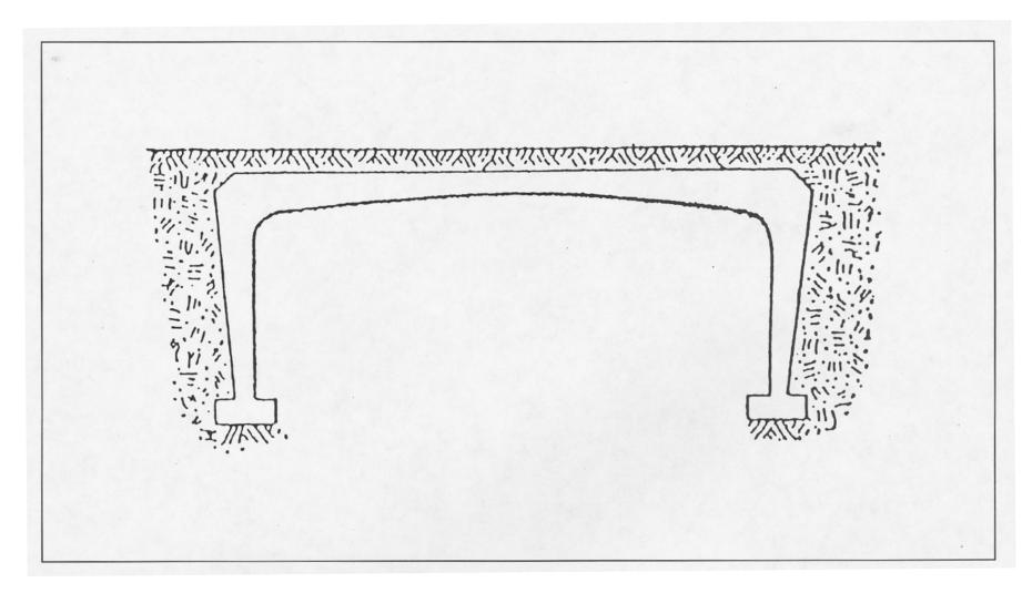
Figure 3.12 Rigid frame structure (Source: Spero 1995: 171).
