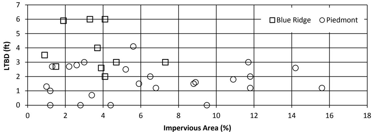
Figure 4.2. LTBD as a function of impervious area.
