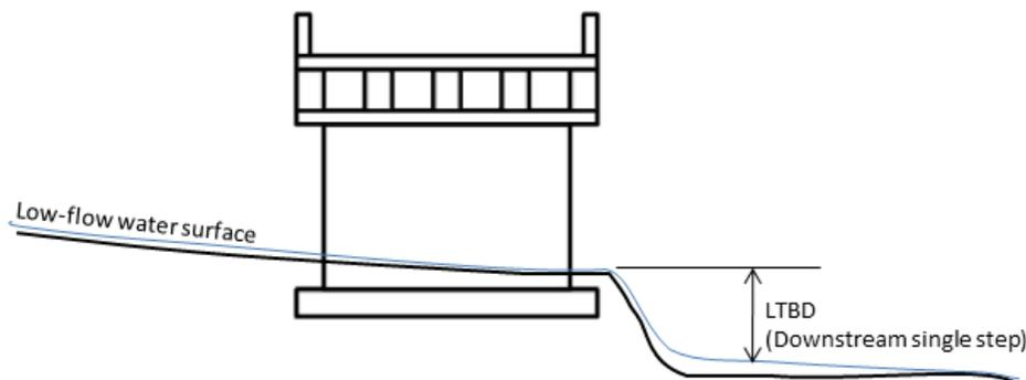
**Figure 3.4.** LTBD: uniform degradation and single step downstream.
