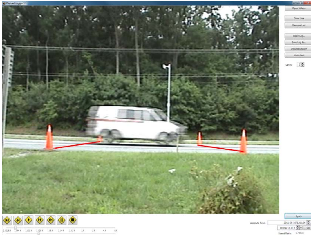
Figure 4-3: Vehicle detection that triggered an all-red phase extension
