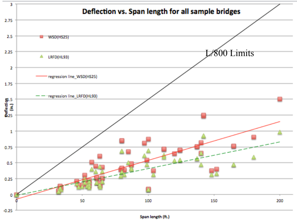
Figure 5.2 Deflection vs. Span Length for All Sample Bridges
