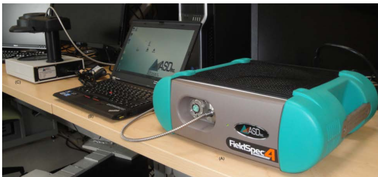
Figure 2. ASD FS4 Setup: (A) – FS4, (B) – Computer Control, and (C) – ASD Turntable.
