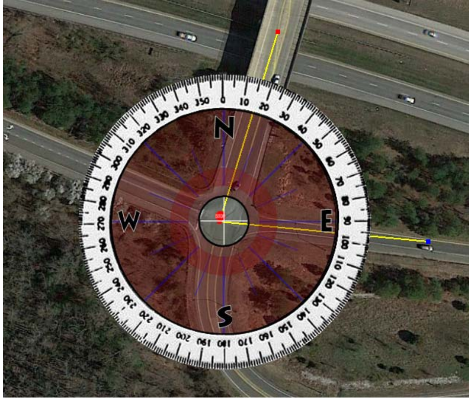
Figure 32. An Example of Exit Ramp Skew Angle Estimation in Google Earth
