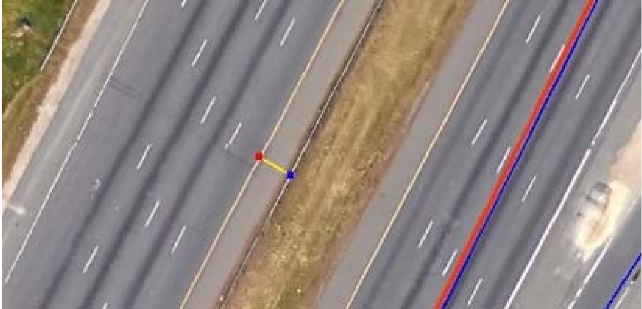
Figure 28. An Example of Median Barrier Offset Measurement
