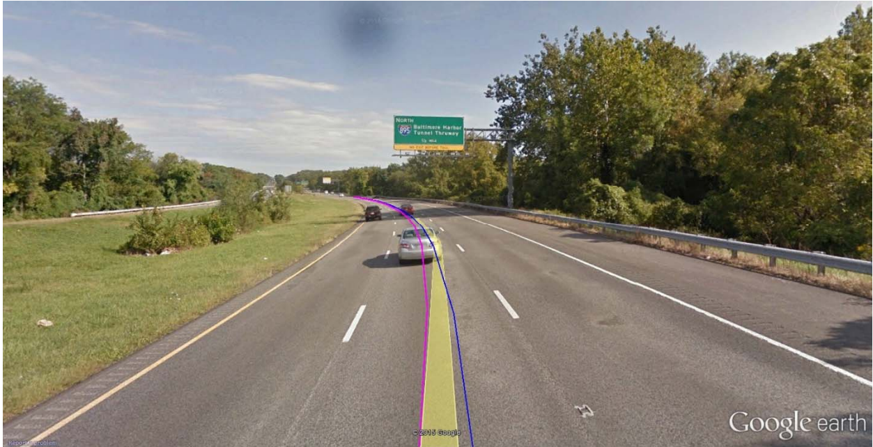
Figure 31. An Example of Identification of Rumble Strips in Google Earth StreetView
