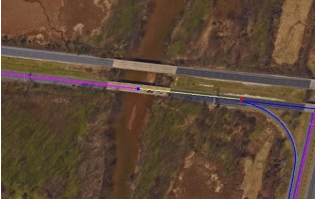
Figure 30. An Example of Distance to Closest Ramp Measurement
