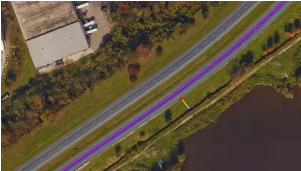
Figure 29. An Example of Outside Clear Zone Width Measurement
