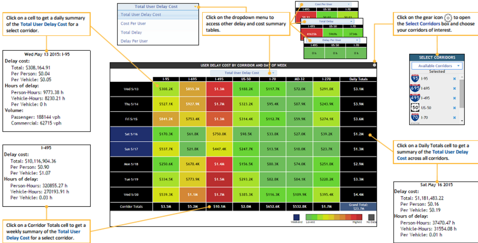
Figure 31: An overview of the work zone dashboard (User Delay Cost by Corridor and Day of Week)
