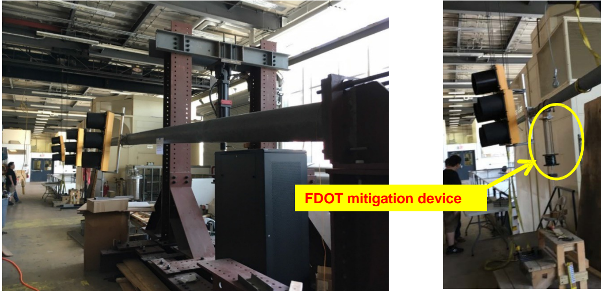
Figure 5.1 - Damping test conducted at the University of Maryland
