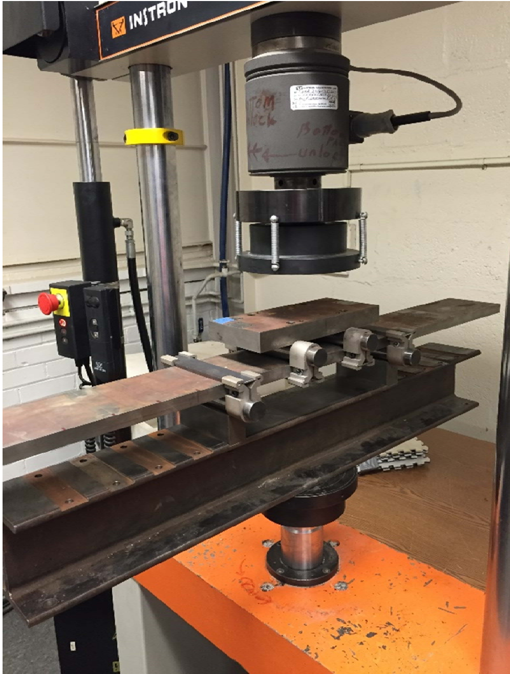
Figure 2-5. Measurement of BVT static stiffness ( k_s ) with the Instron machine.
