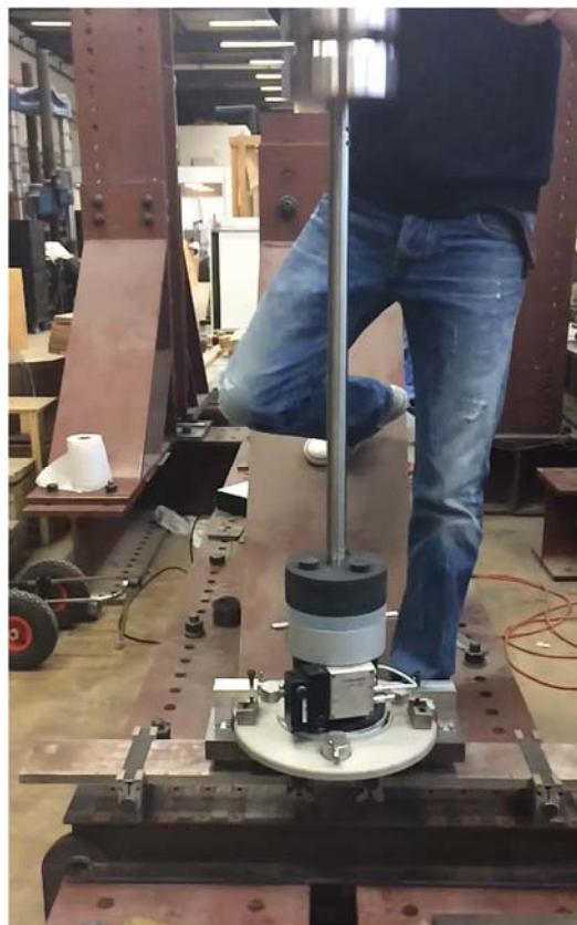
Figure 2-3. Dynatest LWD test performed on BVT
