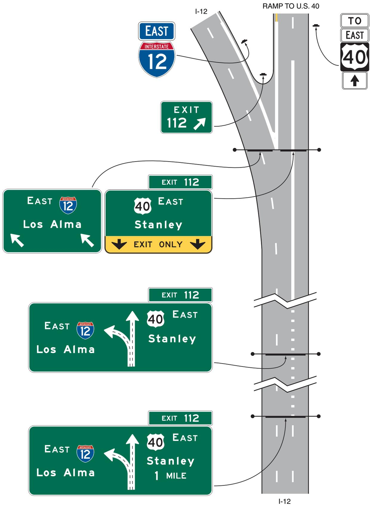
Figure 2E-10. Diagrammatic Guide Signs for a Split with an Option Lane
