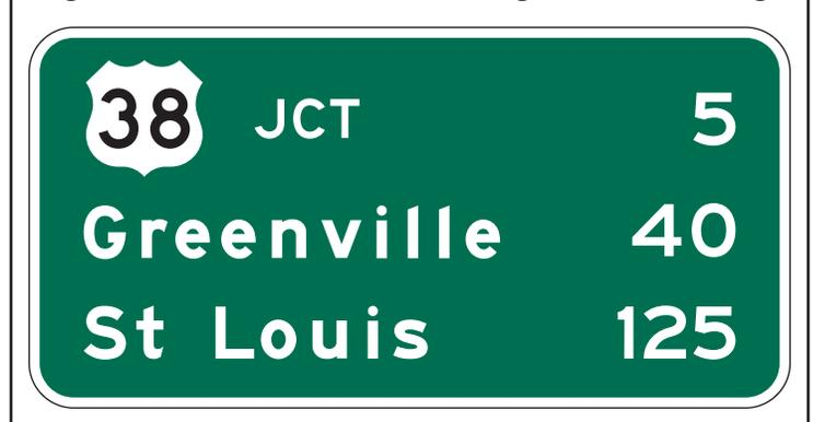
**Figure 2E-30. Example of Using an Interchange Sequence Sign for Closely-Spaced Interchanges**
