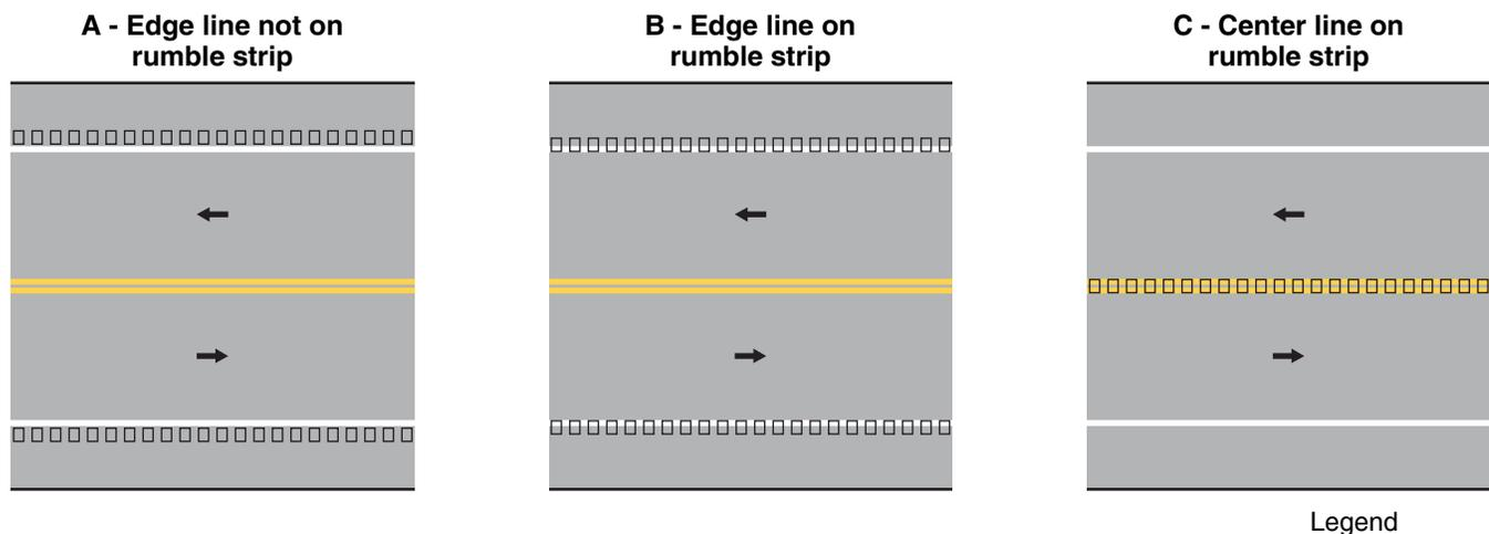
Note: Edge line may be located alongside the rumble strip (Option A) or on the rumble strip (Option B). Center line markings may also be located on a center line rumble strip (Option C).
