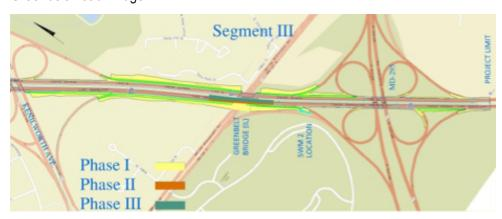
**Phase I** - Compress travel lanes to 11', place TCB, perform utility relocations, construct outside road widening and outside of Greenbelt Road Bridge.
