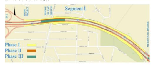
**Phase I** - Compress travel lanes to 11', place TCB, perform utility relocations, construct outside road widening and outside of Rhode Island Ave Bridge.
