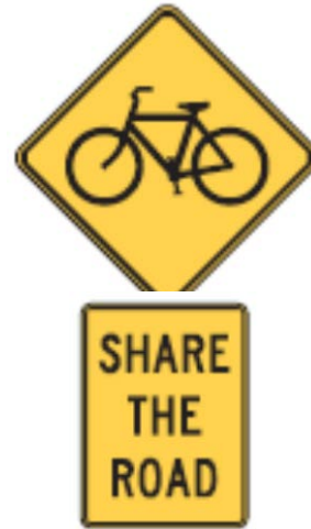
Figure 3.5 SHARE THE ROAD assembly W11-1 and W16-1
