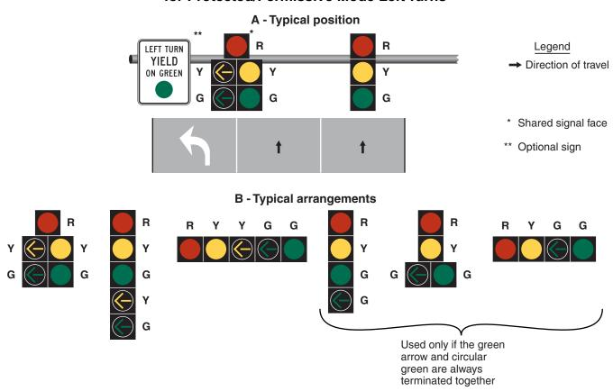
Figure 4D-12. Typical Position and Arrangements of Separate Signal Faces with Flashing Yellow Arrow for Protected/Permissive Mode and Protected Only Mode Left Turns
