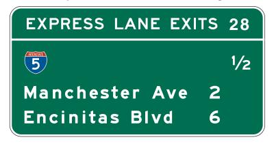
Figure 2G-20. Example of an Comparative Travel Time Information Sign for Preferential or Managed Lanes
