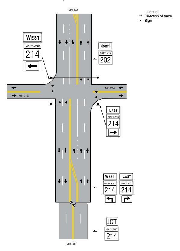
Notes: Confirmation assemblies for north, MD 202 straight ahead may be added with the directional assembly when engineering study determines a need.
