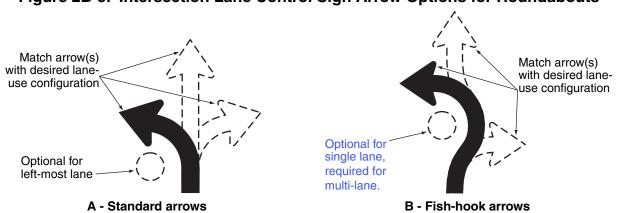
When lane control signs are installed at approaches to State owned, operated, and maintained roundabout intersections, the fish-hook style arrows shall be used.
