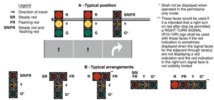
Note: A flashing red arrow controlling a right-turn movement may be used only when an engineering study determines that each and every vehicle must successively come to a full stop before making a permissive turn
