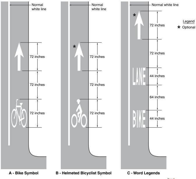
When required, Option A shall be used on State owned, operated, and maintained roadways.
