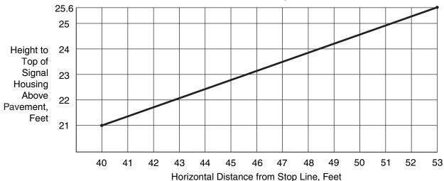
Note: At State owned, operated, and maintained intersections, mounting height of signal faces shall be measured to the bottom of the signal housing to the pavement and shall be a minimum of 17 feet and a maximum of 19 feet.
