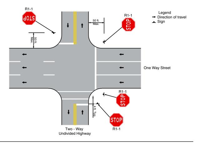
Figure 2B-1b. Example of STOP Signs Placement at "T" Intersection
