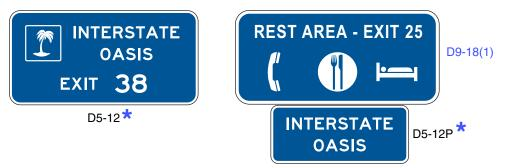
★ Sign shall not be used along State owned, operated and maintained roadways.
