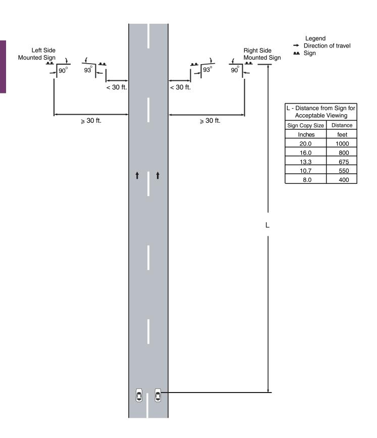
Figure 2A-4b Examples of Clearing Foliage for Sign Installation
