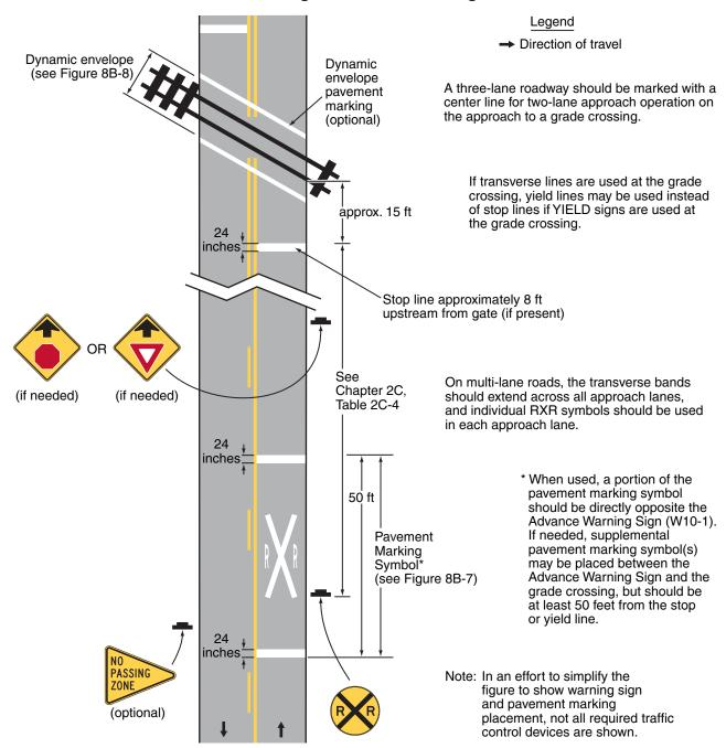
Identical markings shall be placed in each approach lane on all paved approaches to grade crossings where signals or automatic gates are located, and at all other grade crossings where the posted or statutory highway speed is 40 mph or greater.
