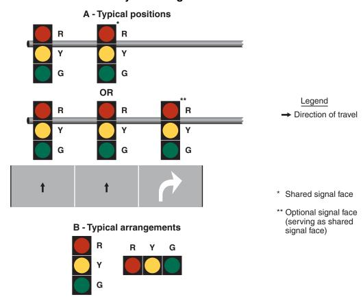
Figure 4D-14. Typical Position and Arrangements of Separate Signal Faces with Flashing Yellow Arrow for Permissive Only Mode Right Turns
