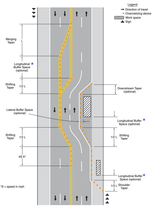
★ Except in cases determined to be impractical or infeasible, a buffer space shall be provided in TTC zones along SHA owned, operated, and maintained roadways.
