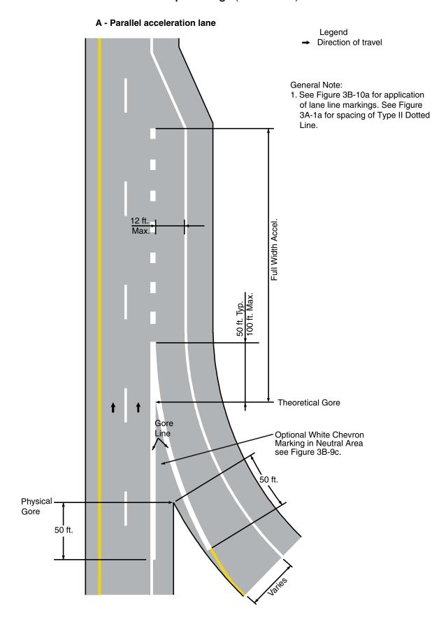
Figure 3B-9. Examples of Dotted Line and Channelizing Line Applications for Entrance Ramp Markings (Sheet 2 of 6)
