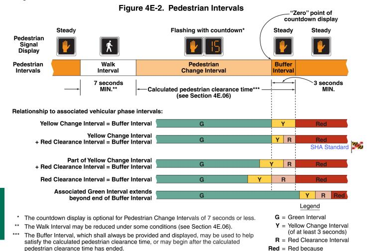
The additional time provided by an extended pushbutton press to satisfy pedestrian clearance time needs may be added to either the walk interval or the pedestrian change interval.
