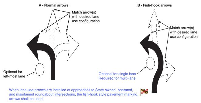
Figure 3C-3. Example of Markings for a One-Lane Roundabout
