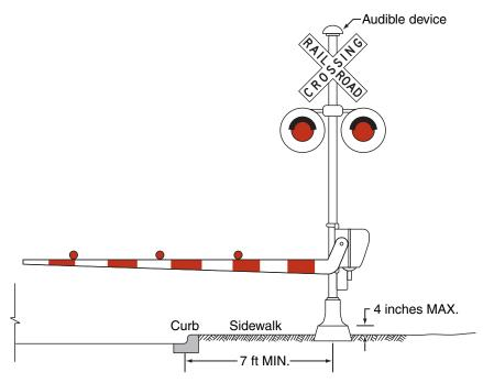
Figure 8C-6. Example of a Separate Pedestrian Gate
