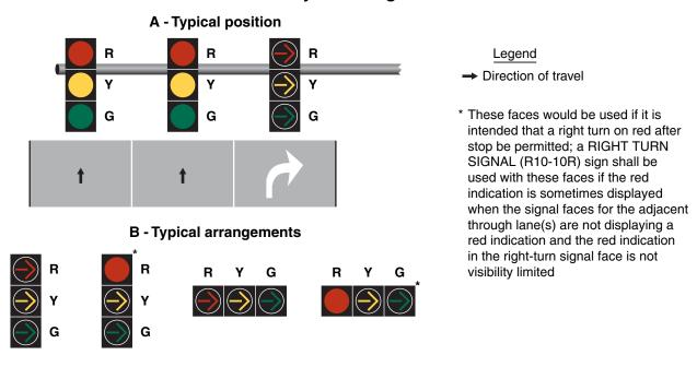
Figure 4D-18. Typical Positions and Arrangements of Shared Signal Faces for Protected/Permissive Mode Right Turns
