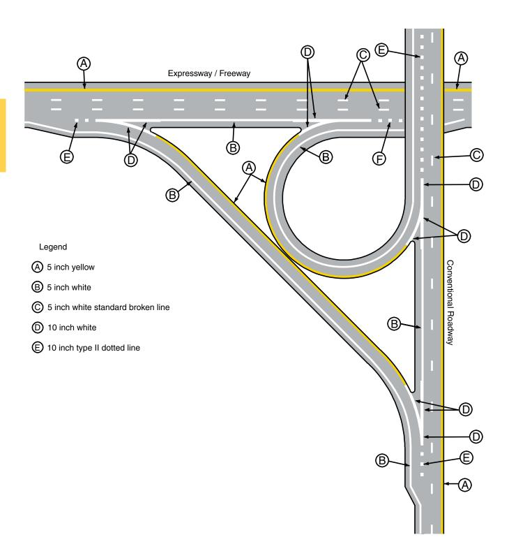
Figure 3B-11. Examples of Applications of Conventional Road Lane-Drop Markings (Sheet 1 of 2)
