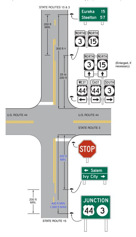
Note: The spacings shown on this figure are for rural intersections. See Sections 2D.29, 2D.30, 2D.32, 2D.34, 2D.40, and 2D.42 for low-speed and/or urban conditions.
