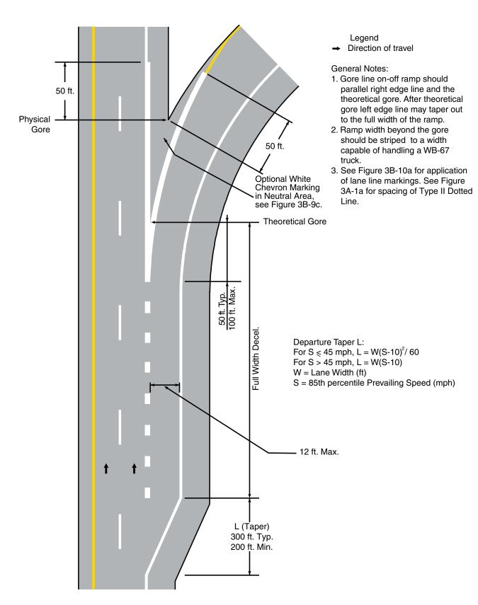
Figure 3B-8. Examples of Dotted Line and Channelizing Line Applications for Exit Ramp Markings (Sheet 2 of 6)
