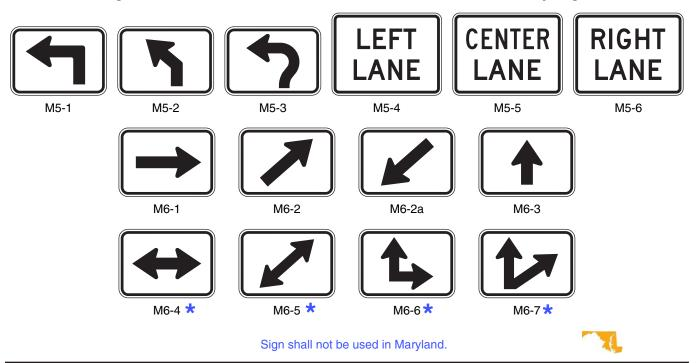
Figure 2D-5a. Examples of Advance Turn and Directional Auxiliary Arrows
