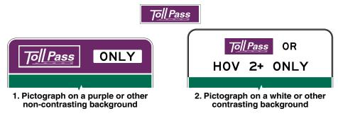
height of the pictograph. When the pictograph is the principal legend on the sign, such as for advance guide signs for open-road tolling lanes (see Section 2F.15), the minimum height of a horizontal rectangular ETC pictograph should be consistent with that of a route shield prescribed for the particular application and type of sign.
