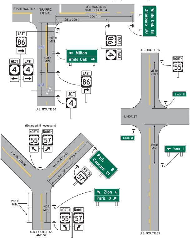
Note: The spacings shown on this figure are for rural intersections (400 ft < L ≤ 1,000 ft). See Sections 2D.29, 2D.30, 2D.32, 2D.34, 2D.40, and 2D.42 for low-speed and/or urban conditions.
