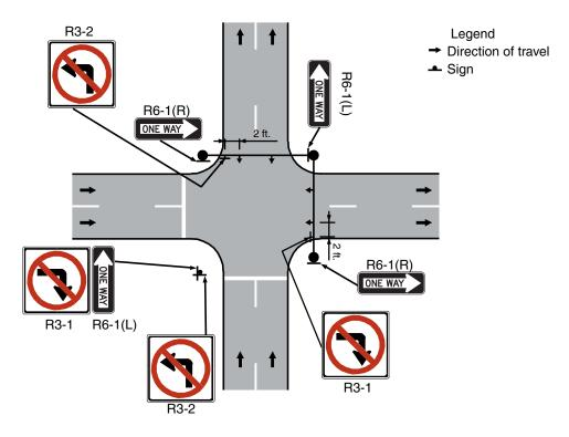
Figure 2B-4e. Example of NO LEFT TURN Signs Placement at a Signalized Intersection, Divided Highway
