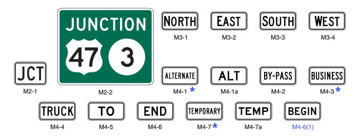
★ Sign shall not be used along State owned, operated and maintained roadways.
