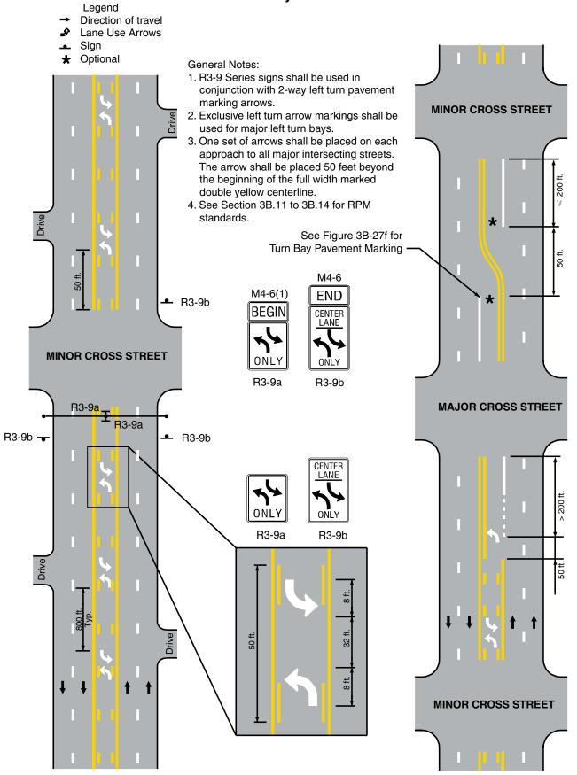
Figure 3B-7b. Examples of Left Turn Lane with Two-way Center Left Turn
