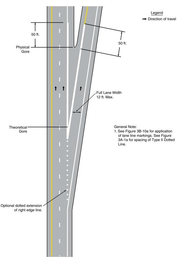
Figure 3B-8. Examples of Dotted Line and Channelizing Line Applications for Exit Ramp Markings (Sheet 4 of 6)
