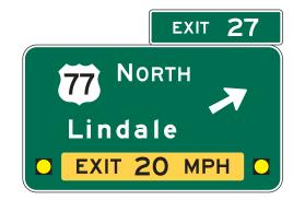
Exit Direction sign with E13-2 sign panel and flashing yellow beacons
