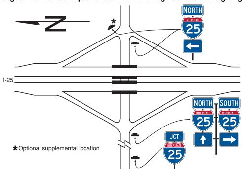
Figure 2D-12. Example of Minor Interchange Crossroad Signing
