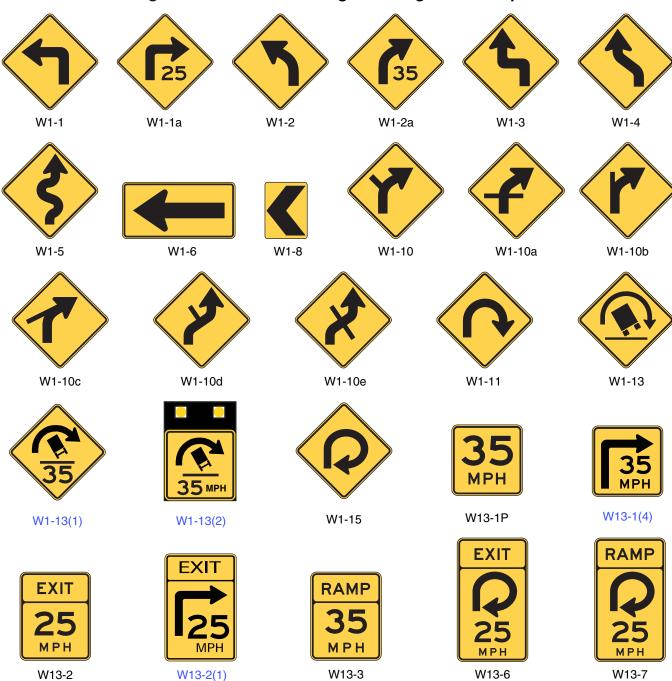
Note: Turn arrows and reverse turn arrows may be substituted for the curve arrows and reverse curve arrows on the W1-10 series signs where appropriate.
