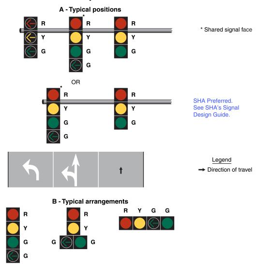
Note: Shared signal faces shall only be used for a protected-only mode left turn if the circular green and green left-turn arrow indications always begin and terminate together
