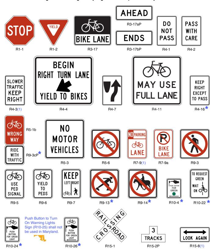
\* Sign shall not be used along State owned, operated and maintained roadways.
