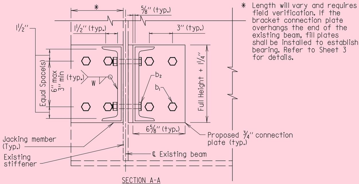
\* Length will vary and requires field verification. If the bracket connection plate overhangs the end of the existing beam, fill plates shall be installed to establish bearing. Refer to Sheet 3 for details.
