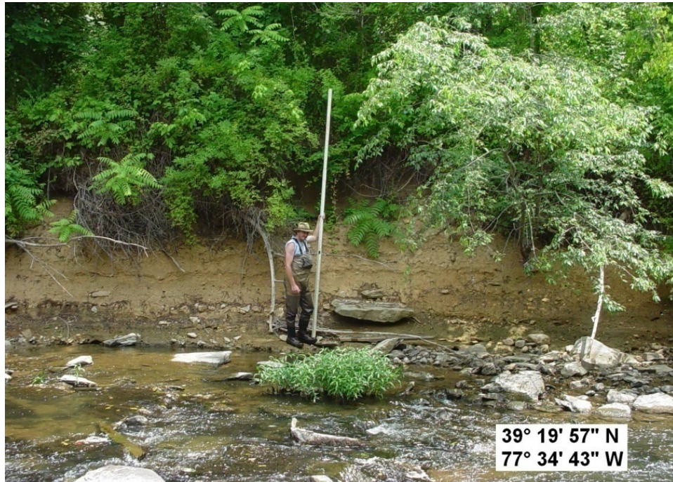
Photo 70: Left bank height (11') between MD 464 Bridge and existing bridge abutment. This vertical bank is composed of legacy sediments and is typical of the banks found throughout the site.
