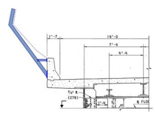
Construct a physical barrier on the outside face of the existing bridge parapet to lean away from the bridge so as not to encroach on the shoulder of the bridge where it could be struck by a vehicle. Lean the barrier away from the bridge at a slope that would make it difficult to climb. Netting could be used between posts rather than a fence-type material.
