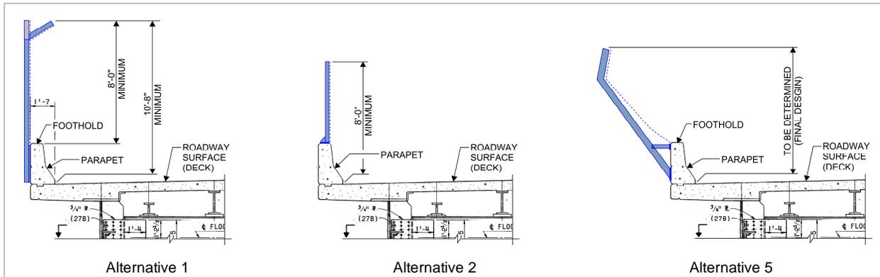
**Figure 5. Alternatives 1, 2, & 5 (Barrier) Conceptual Sketches**
