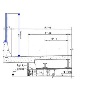
Construct a physical barrier on top of the existing concrete parapet. The geometry of the new barrier would be developed to not encroach on the shoulder of the bridge where it could be struck by a vehicle. The barrier will be designed and detailed such that there would be no additional stepping-point above the roadway surface and therefore the new barrier can be measured from the roadway surface. This would likely result in an overall shorter barrier than Alternative 1.
