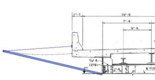
Construct netting on the outside of the bridge and located at or near the level of the bridge roadway surface.
