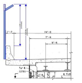
Construct a physical barrier on the outside face of the existing parapet, while retaining the existing parapet. Since the existing parapet could be used as a stepping point to climb the new barrier, the height of the new barrier will be referenced from the top of the existing parapet. The geometry of the new barrier will be developed to not encroach into the shoulder of the bridge where it could be struck by a vehicle.
