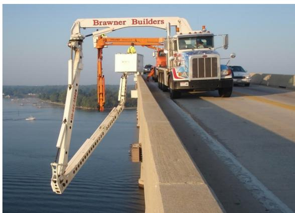
Figure 8. Under-Bridge Inspection Vehicle
