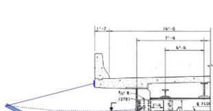
Construct netting on the outside of the bridge and located below the bridge roadway surface.
