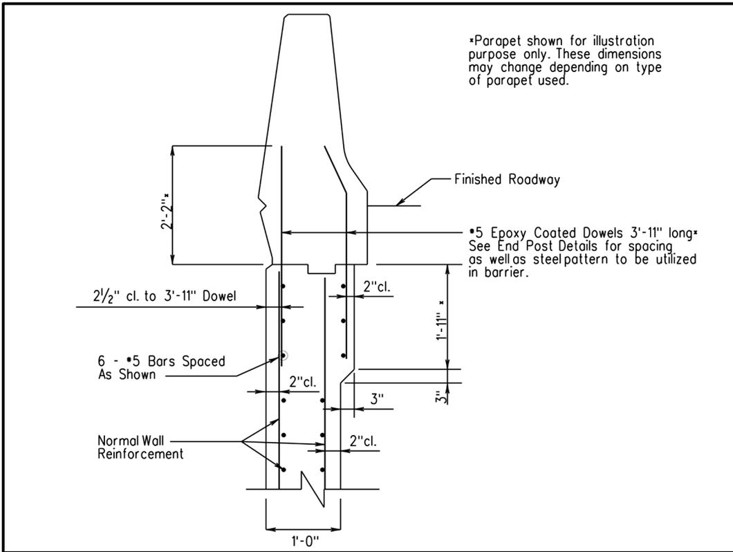
Figure 2-7: Parapet Attachment for Walls with 1'-0" Stem Thickness
