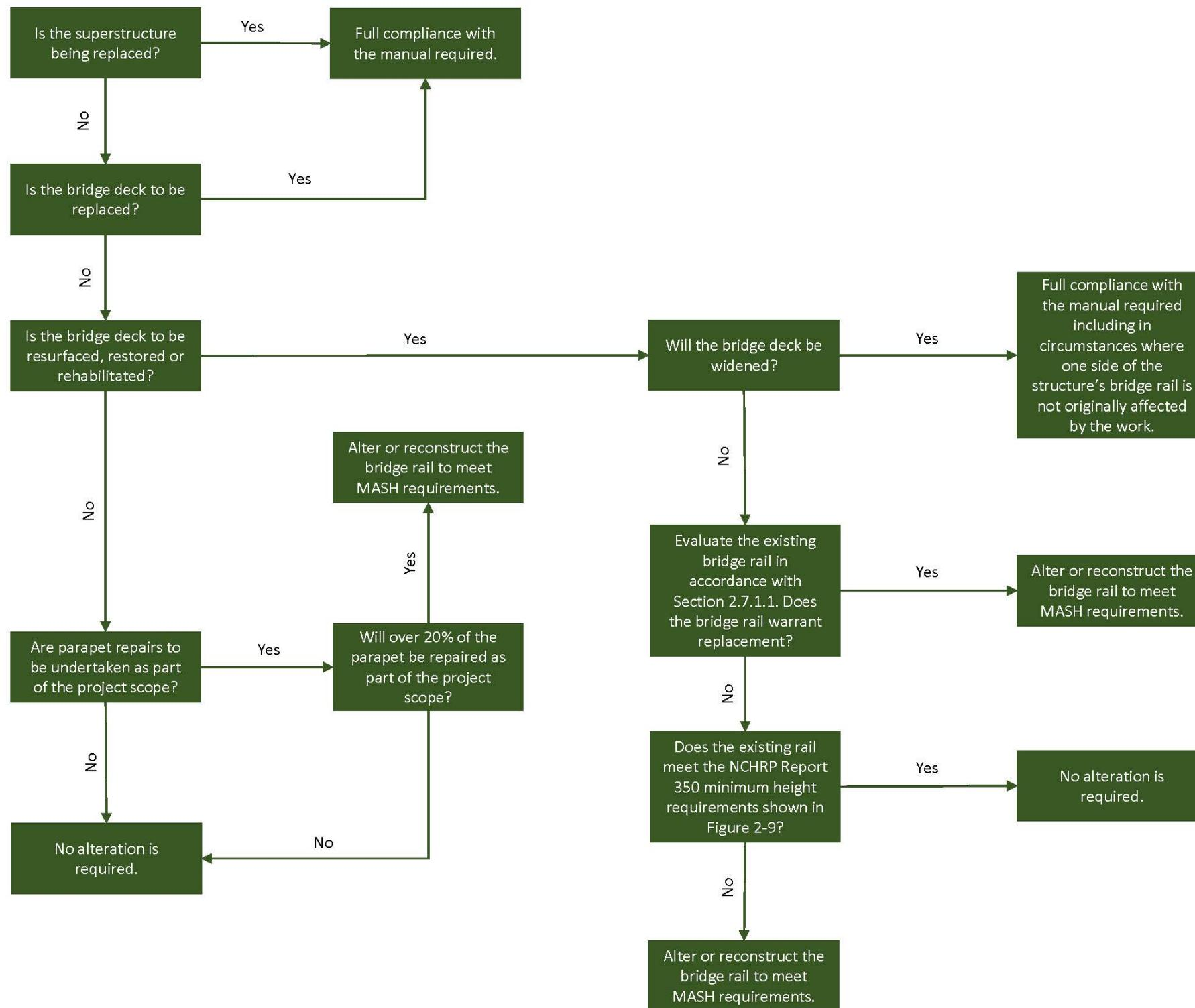
Figure 2-10: Treatment of Existing Bridge Rail
