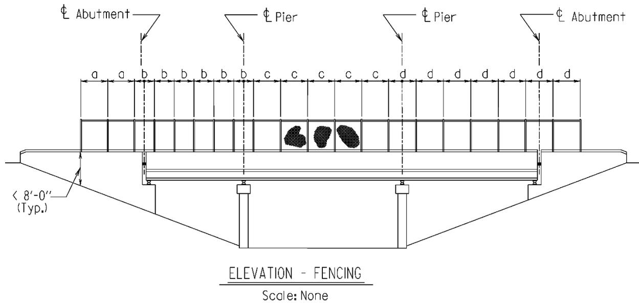
Figure 2-6: Fence Spacing on Bridges
