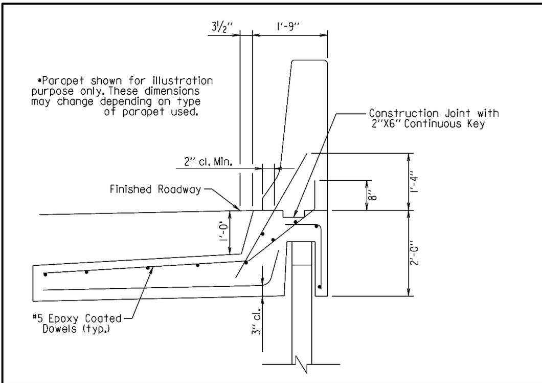
Figure 2-8: Barrier Doweled into Moment Slab
