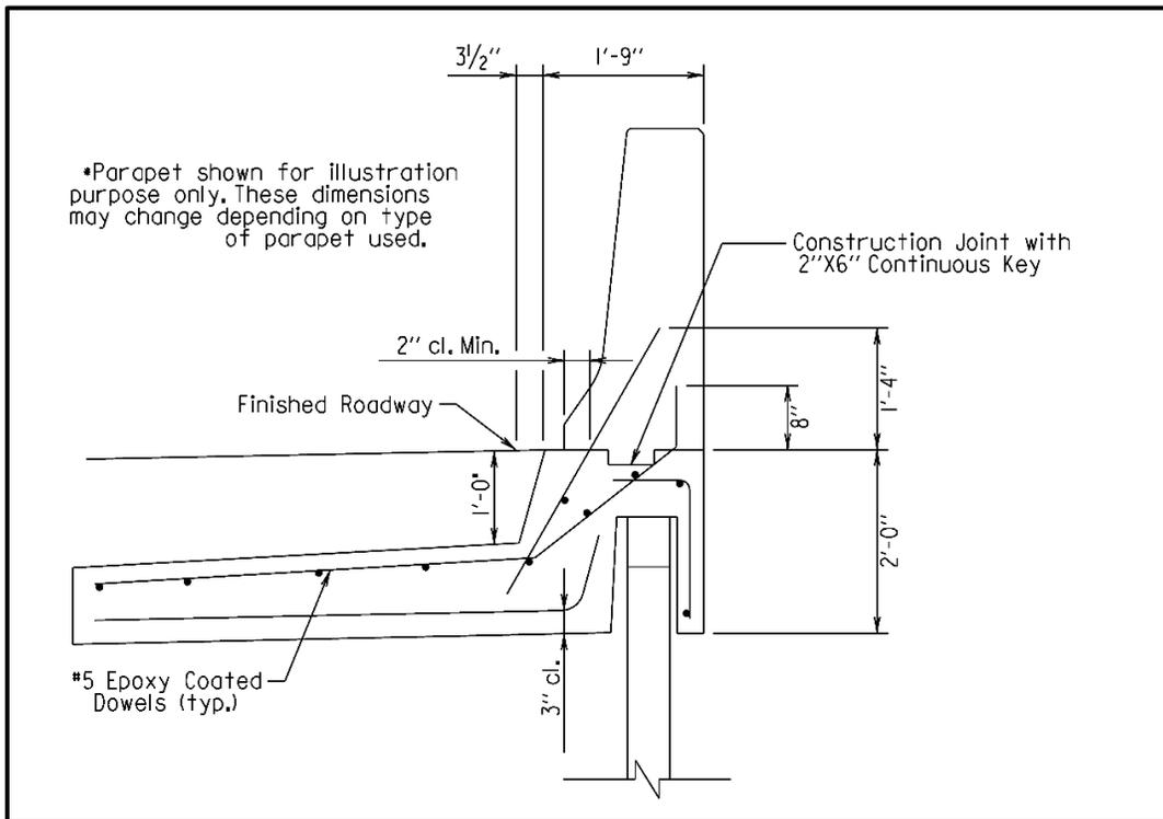
Figure 2-8: Barrier Doweled into Moment Slab
