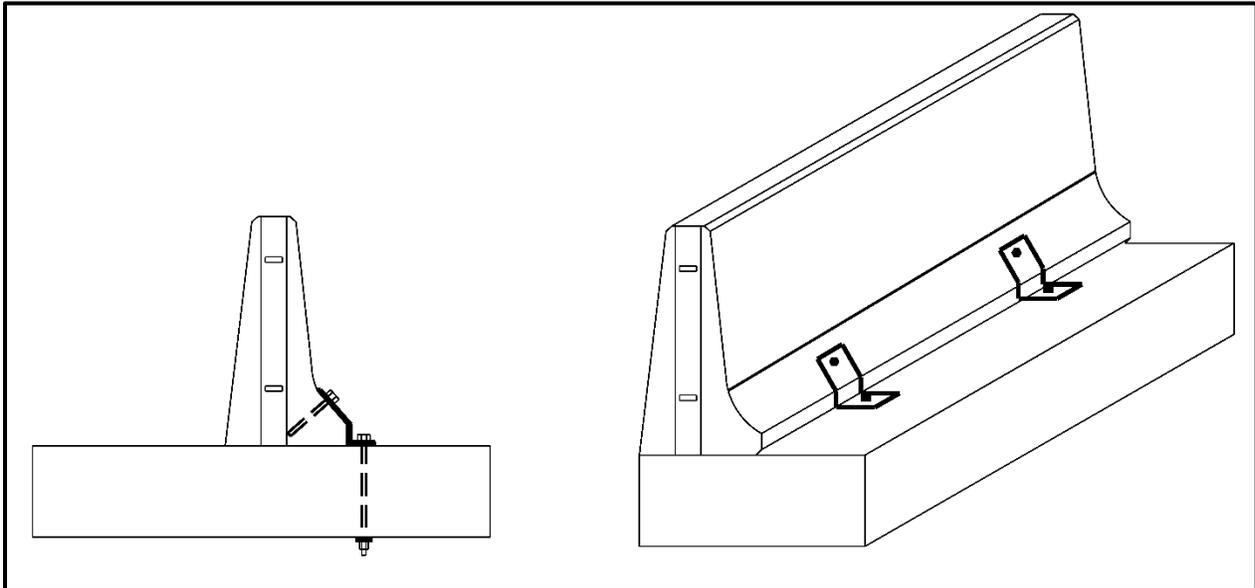
**Low Deflection Pinned to Concrete Bridge Deck (MOT-101)**
