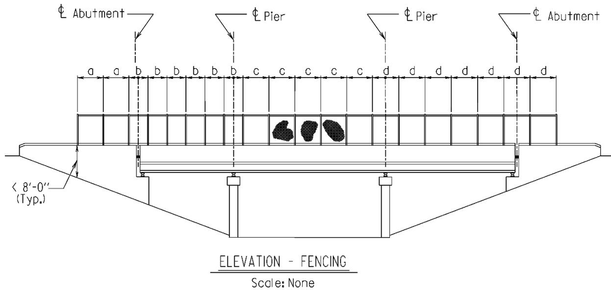
Figure 2-6: Fence Spacing on Bridges
