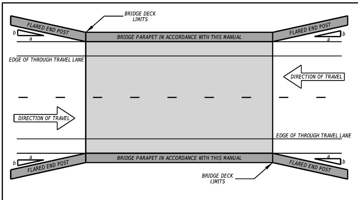
Figure 2-4: Tapered End Posts at Locations where Aesthetics is a concern and there is no Adjacent Traffic barrier
