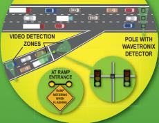
INTELLIGENT SIGNAL SYSTEMS optimize traffic flow onto I-270
