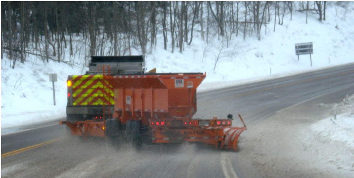
The tow plow unfolds to the side, allowing the driver of a single truck to plow two lanes.
