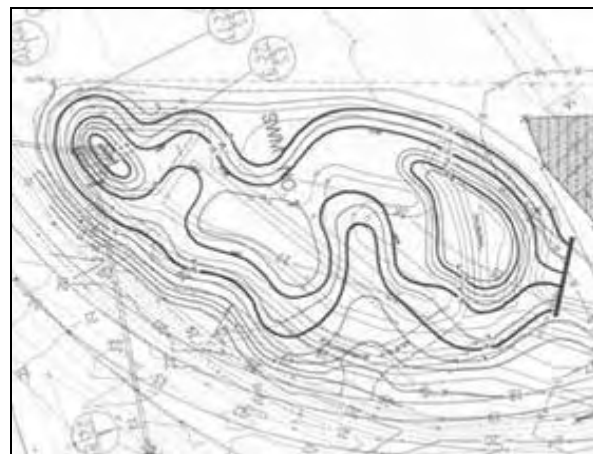
Figure 3-8 Comparison of Square versus Curvilinear BMP Design (from VEQ-S Reviewer Guidelines)
