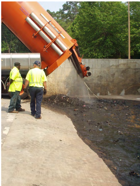
Vacuum Truck at Owings Mills Shop Dewatering Facility
