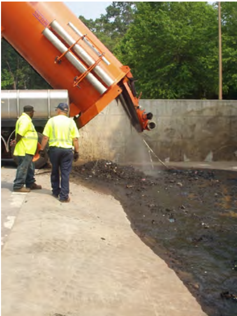
Figure 1-14: Vacuum Truck at Owings Mills Shop Dewatering Facility
