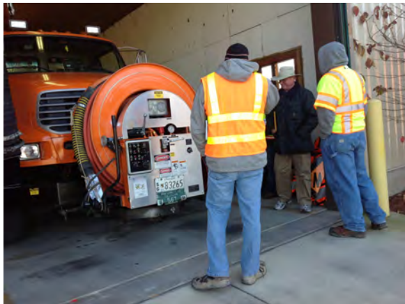
Figure 1-2: EPA Inspection of a Vacuum Truck used for Inlet Cleaning
