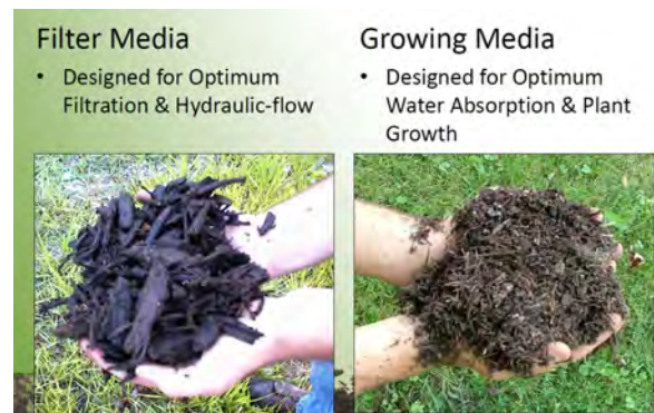
Figure 1-12: SWM Filtration Media with Compost
