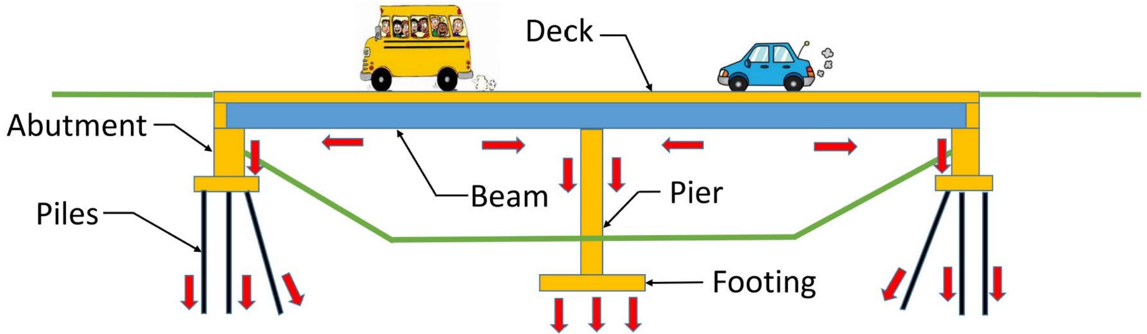
This diagram shows the names for different parts of a bridge. The arrows show how forces are directed between the bridge parts so that the bridge stays standing and supports its loads.
