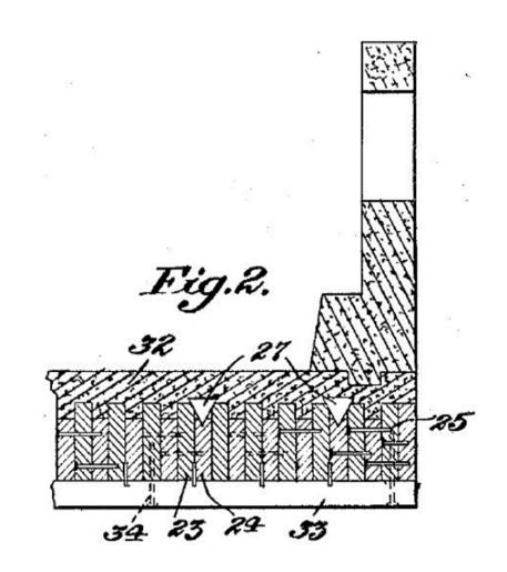
This cross-section detail, from Seiler's patent, shows the two sizes of wood placed in an alternating pattern and covered by concrete. The cross-section also shows a concrete parapet or railing.
