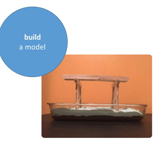
This bridge model example uses the basic bridge deck unit with cross-braced piers constructed with jumbo craft sticks. To simulate the layers of mud found in the soil boring, whipped cream is layered above a denser layer of brownie. You might be able to use sand, gravel, or dirt to simulate the river bottom.
