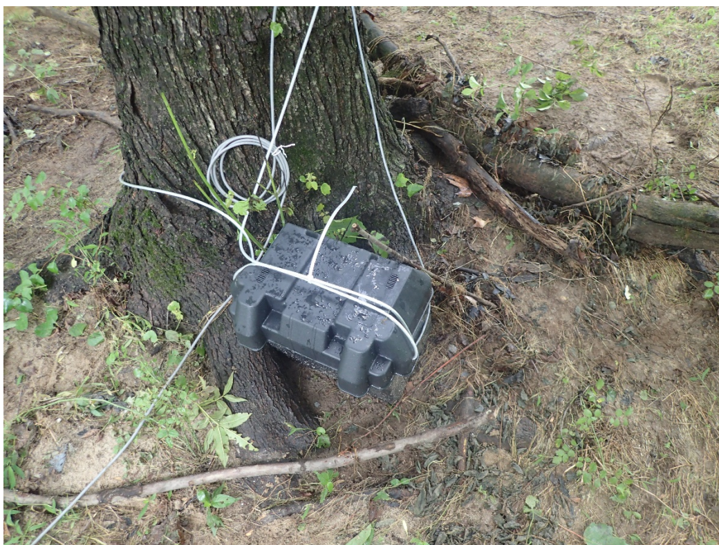
Photograph 30. 6/21/2018: Flow Station 3, area-velocity meter marine battery housing
