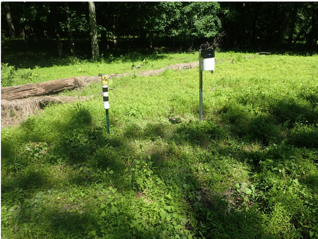
Photograph 12. 6/12/2018: Barometer (left) and rain gauge (right) set-up
