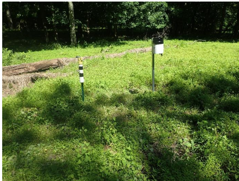
Figure 5. Barometric sensor (left) & rain gauge (right)
