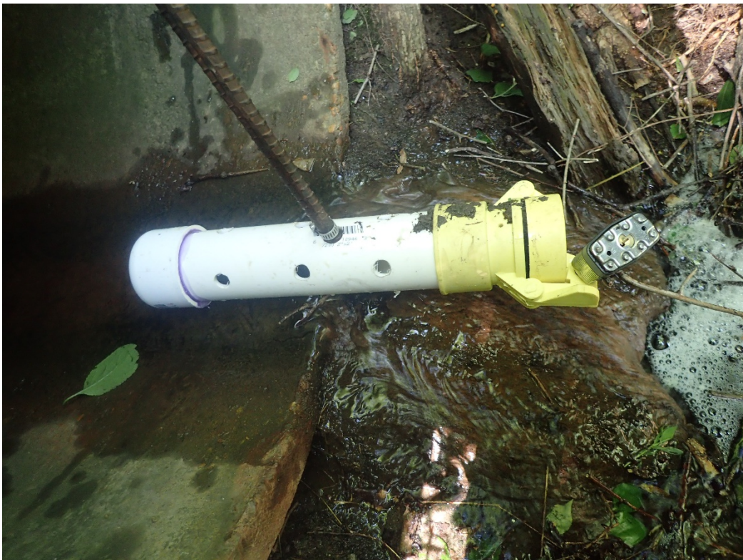
Photograph 6. 6/12/2018: Flow Station 2, depth logger housing
