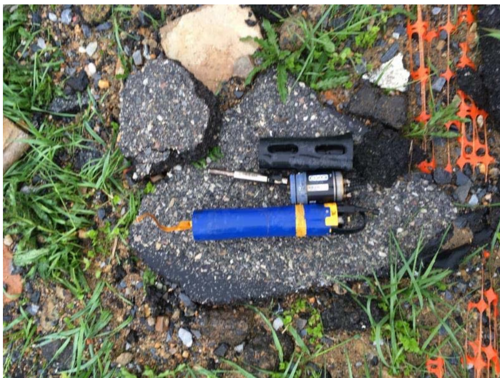
Photo 6 - Remaining components of the EXO2 multiparameter sonde deployed at USGS station 01636845. Attached turbidity probe continued to take observations throughout the event
