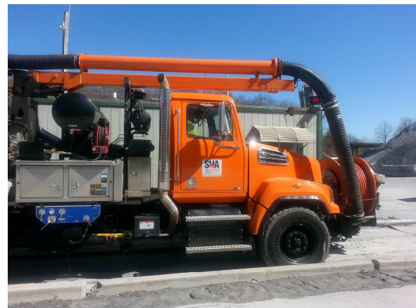
Figure 1-18: MDOT SHA Vacuum Truck Used to Clean Inlets
