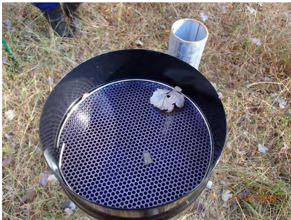
Photograph 58. 11/01/2018: Rain gauge with collected debris, monthly download before maintenance
