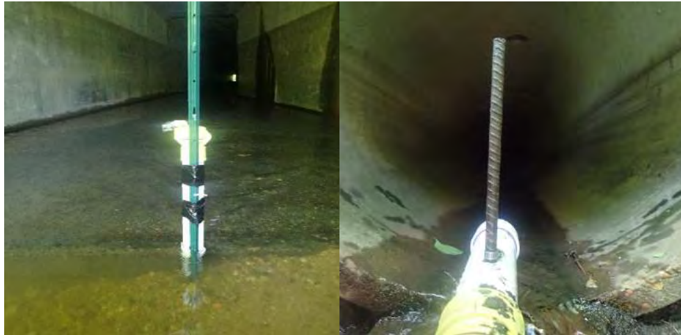
Figure 3. Depth logger mounted at box culvert bottom upstream of I-70 (left; Flow Station 1) and at the outfall of the proposed ESDs (right; Flow Station 2)
