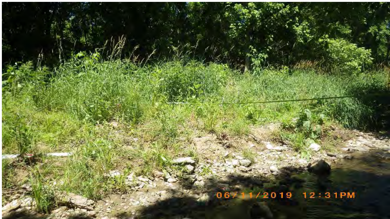
Photo 12 - Cross Section P-6 – Looking at the left, eroded bank with exposed pin – June 2019
