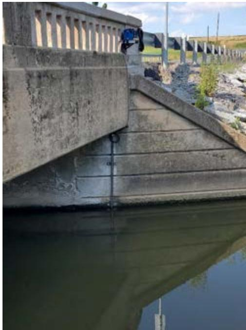
Figure 5. FY22 upstream station (Site ID 01636845) on Little Catocin Creek near Rosemont, MD. The photo shows the ISCO velocity and area flow module.
