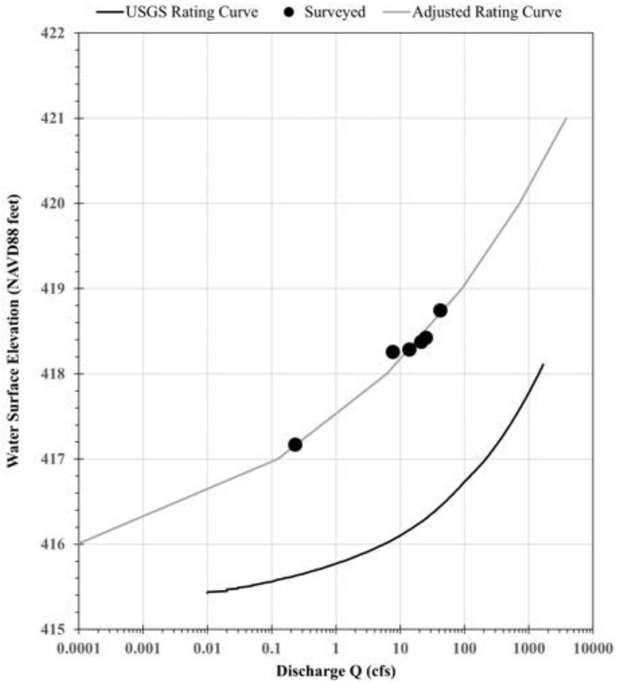
Figure 6. Upstream station (Site 01636845) rating curve
