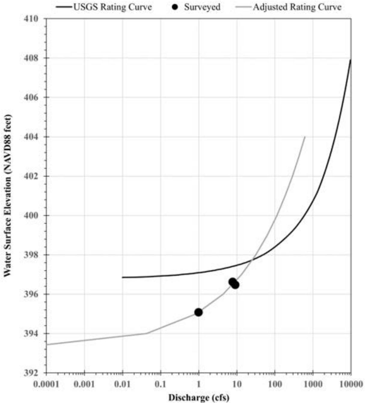
Figure 7. Downstream station (Site 01636846) rating curve
