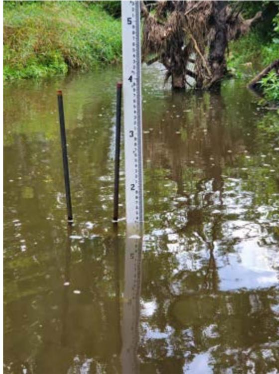
Figure 4. FY22 relocated downstream station (Site ID 01636846) on Little Catocin Creek near Rosemont, MD. The photo shows the HOBOT logger and stream gage.
