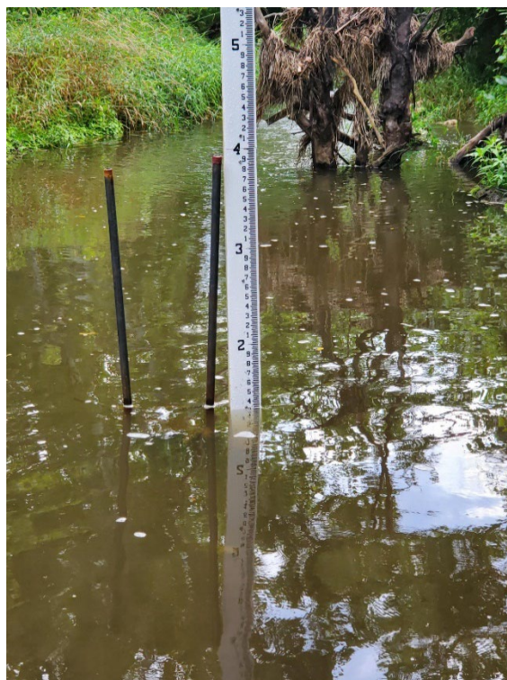
Figure 4. Relocated downstream station (Site ID 01636846) on Little Catoctin Creek near Rosemont, MD. The photo shows the HOBOT logger and stream gage.
