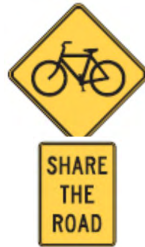
Figure 3.5 SHARE THE ROAD assembly W11-1 and W16-1
