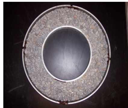
Figure 1- Casting mold and mold with placed aggregate.
