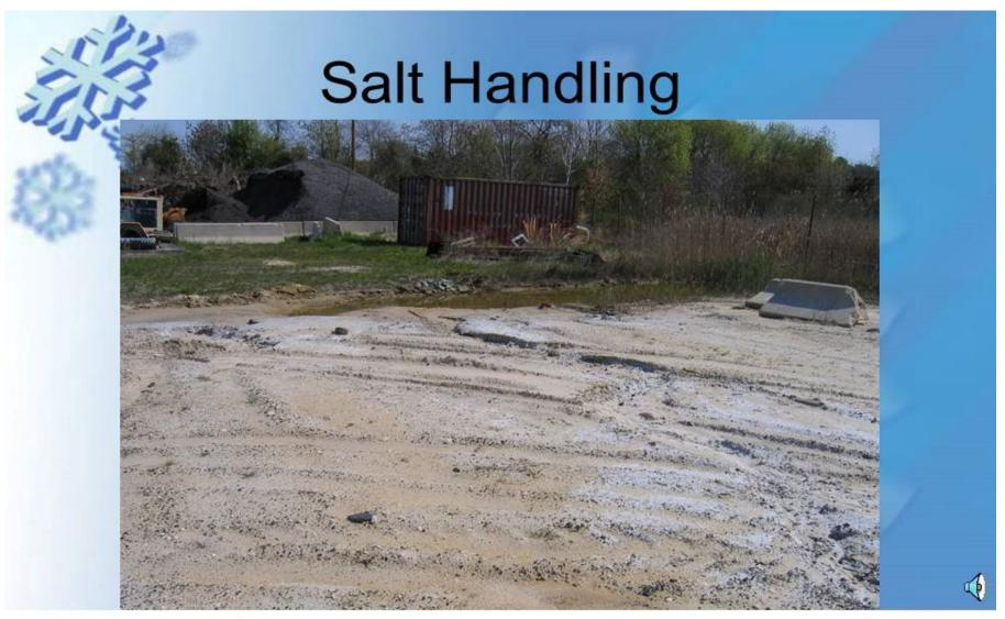
Mixing salt/abrasives on unpaved areas can result in destroying vegetation and causing an erosion problem.
