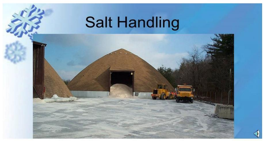
To minimize spillage do not overfill trucks with salt or salt/abrasive mix. Upon completion of plowing event, all material on macadam (pavement) lot must be swept and returned to covered storage.
