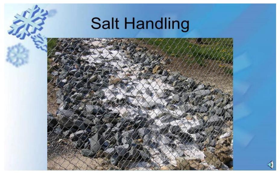
Impact of a salt/abrasive mix not being placed under cover. Non-compliant with NPDES permit conditions.
