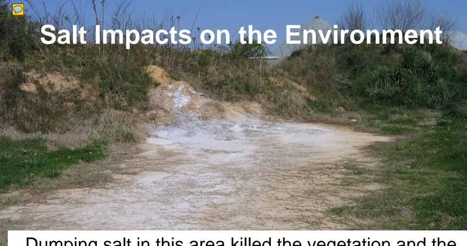
Dumping salt in this area killed the vegetation and the area was at risk for erosion. This area had to be restored by removing contaminated soil, backfilling and seeding and mulching.
