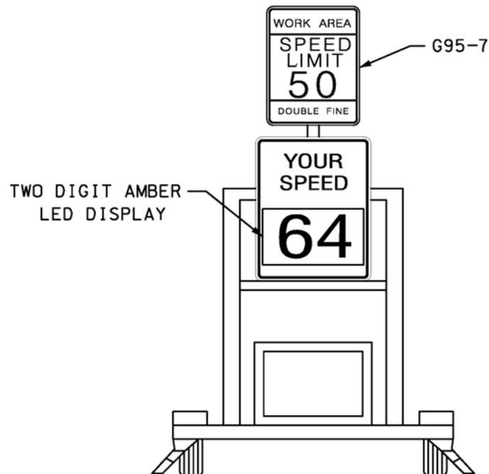
**Figure 2.** Speed display configuration to be used on roadways with lateral restrictions.
