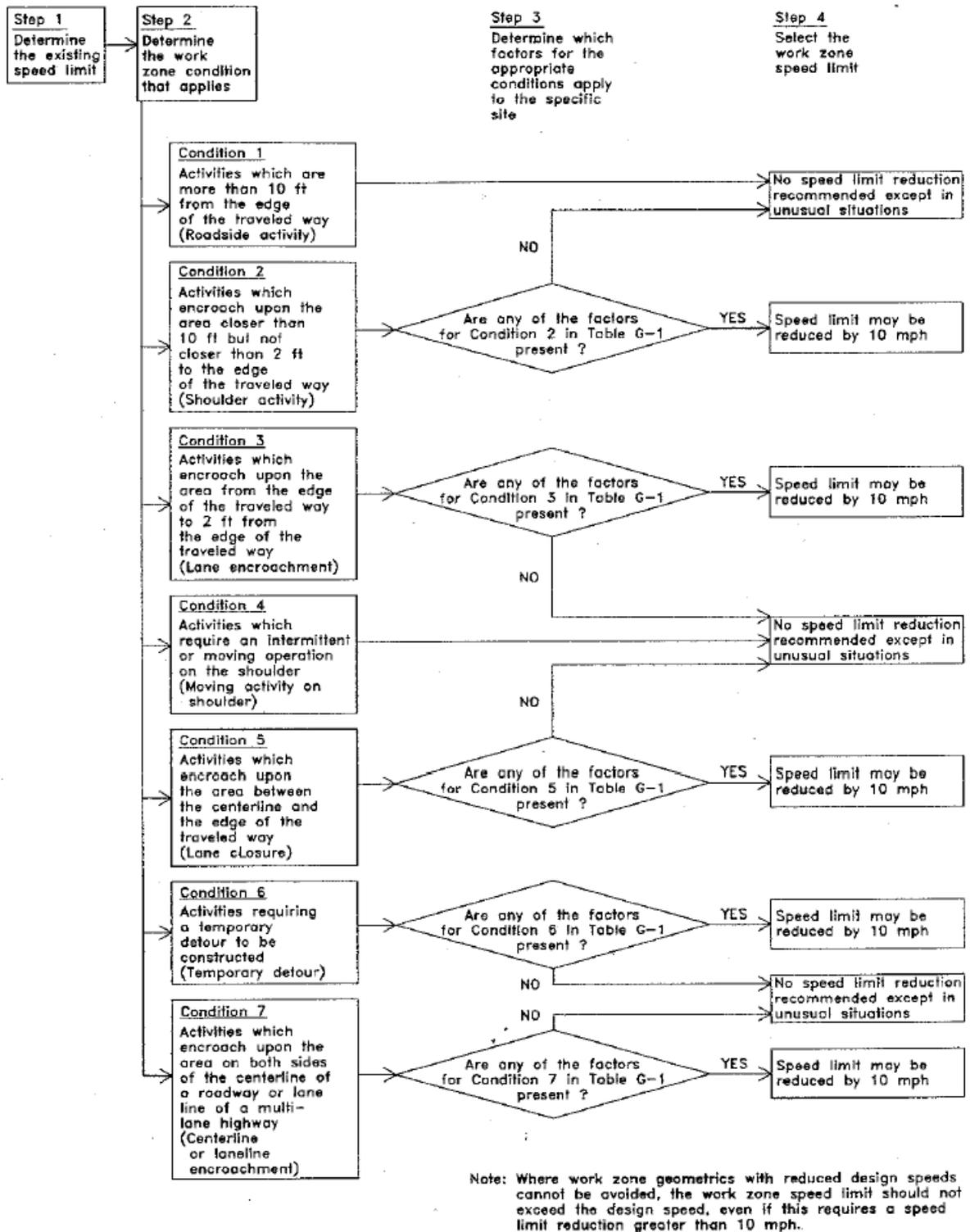
Figure 1. Work zone speed limit procedure flowchart.
