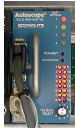
Figure 52 – Video Interface Card (Close Up)
