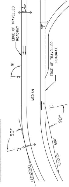
\* UNDER 30 FEET FROM TRAVELLED ROADWAY TO NEAR EDGE OF SIGN - 93° AWAY FROM THE ROAD TO AVOID SPECULAR REFLECTION AS INDICATED IN 813.03 OF THE MARYLAND STANDARD SPECIFICATIONS FOR CONSTRUCTION AND MATERIALS.
