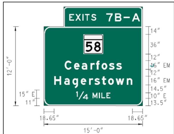
**Figure SN.7 - Final Layout for Design Example**
