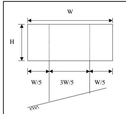
Figure SN.29 - Standard Sign Support Spacing (Two Supports)
