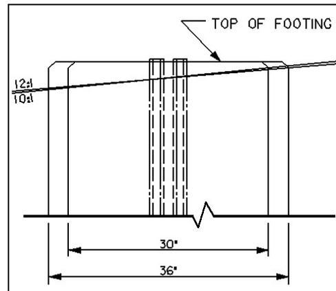
Figure SN.34 - Slope Limits for Foundations
