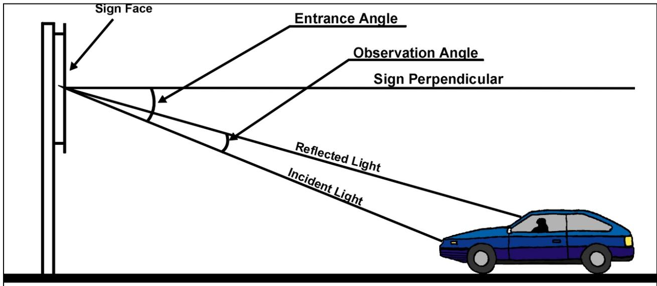
Figure SN.43 - Observation and Entrance Angle (Elevation View)
