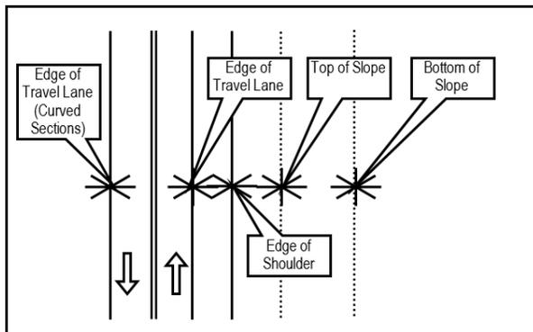
**Figure SN.3 - Typical Elevation Requirements**
