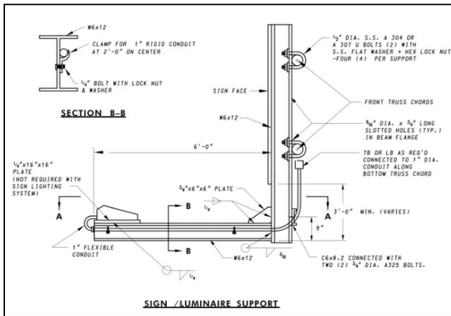
**Figure SN.13 - Sign Lighting Supports**
