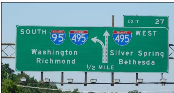
Figure SN.11 - Typical Diagrammatic Sign
