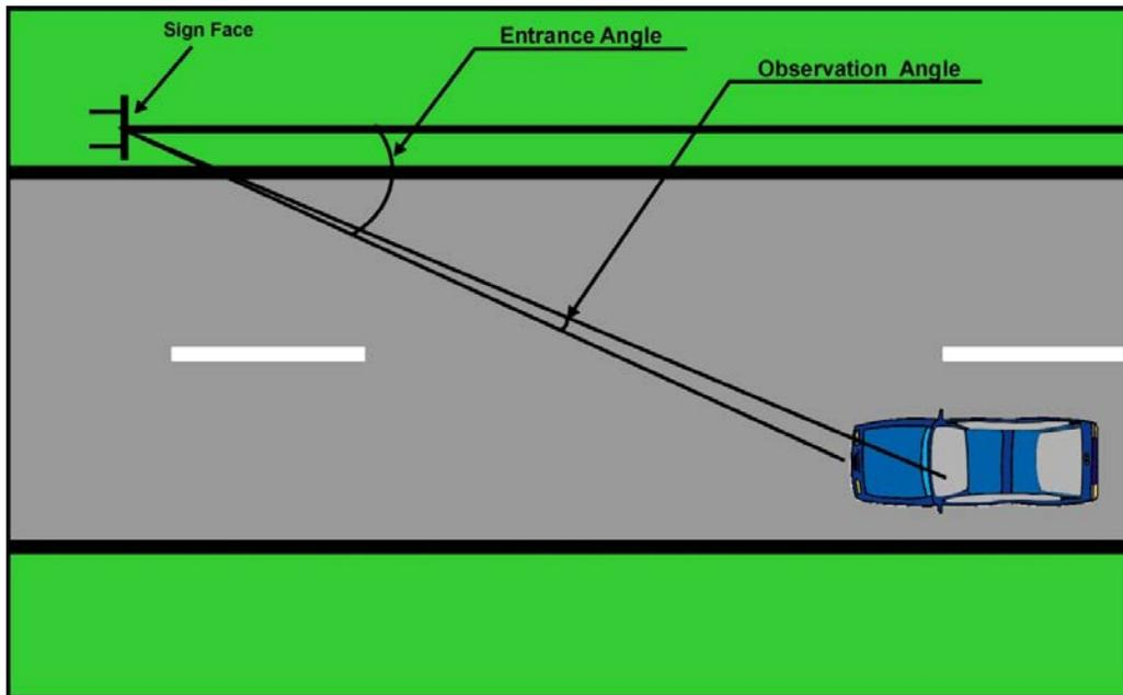
Figure SN. 44 - Observation and Entrance Angle (Plan View)
