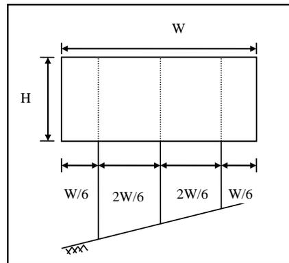
Figure SN.30 - Standard Sign Support Spacing (Three Supports)
