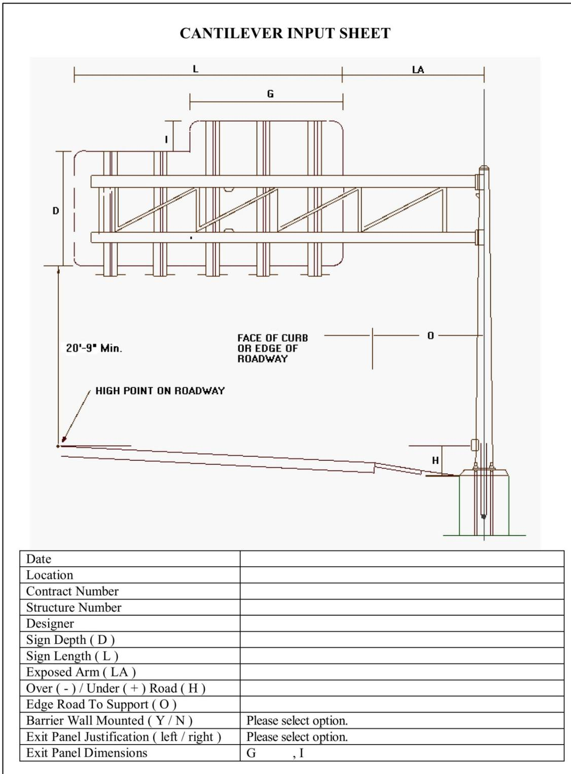
**Figure SN.20 - Structure Input Sheet for New Cantilever Structures**
