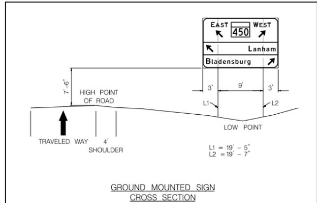
**Figure SN.22 - Example of a Cross Section for Determining Sign Support Lengths**
