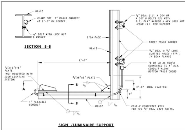
**Figure SN.13 - Sign Lighting Supports**
