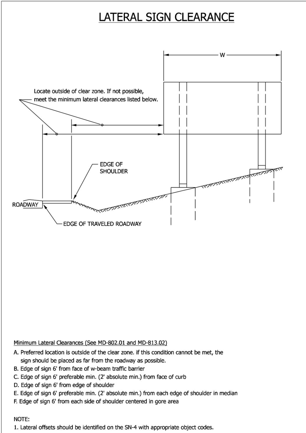
**Figure SN.42 - Lateral Sign Clearance**
