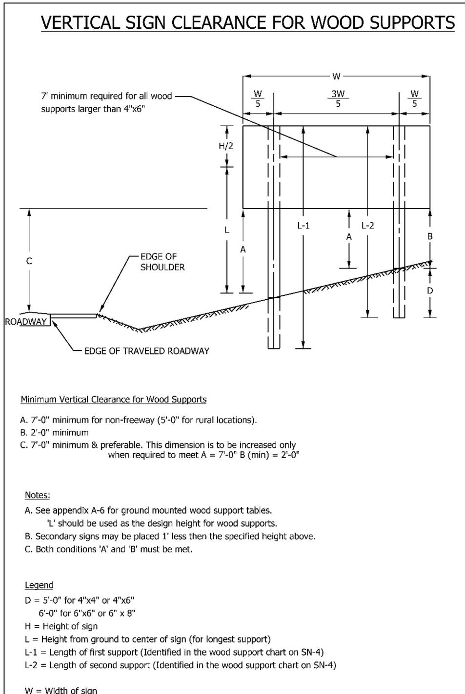
Figure SN.27 - Wood Support Vertical Clearance
