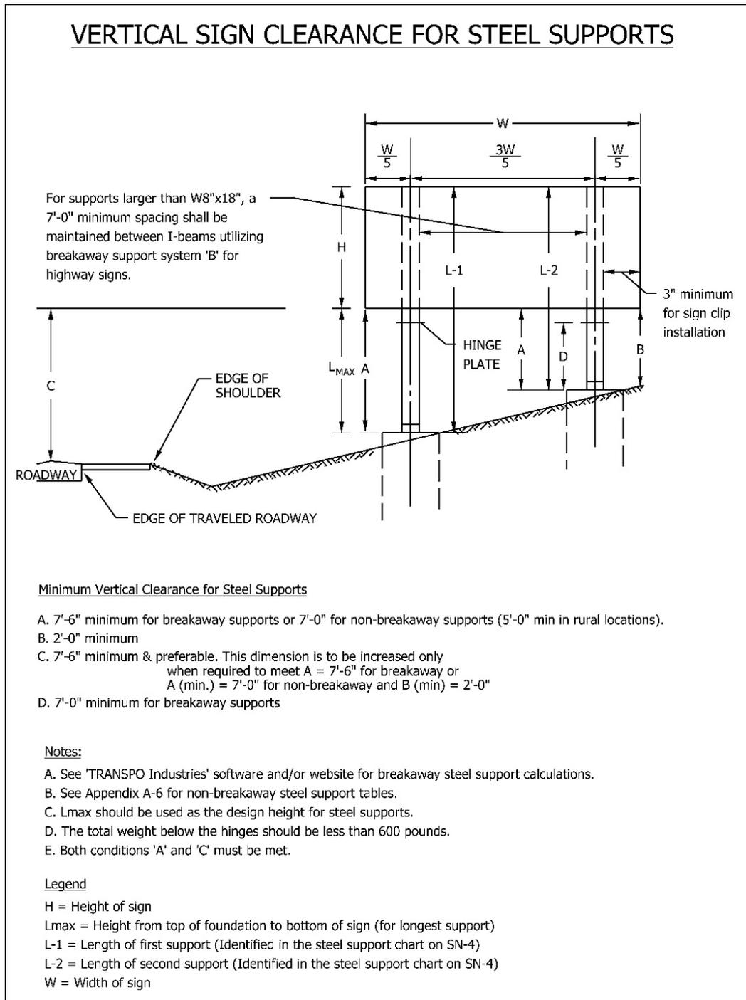
Figure SN.28 - Steel Support Vertical Clearance
