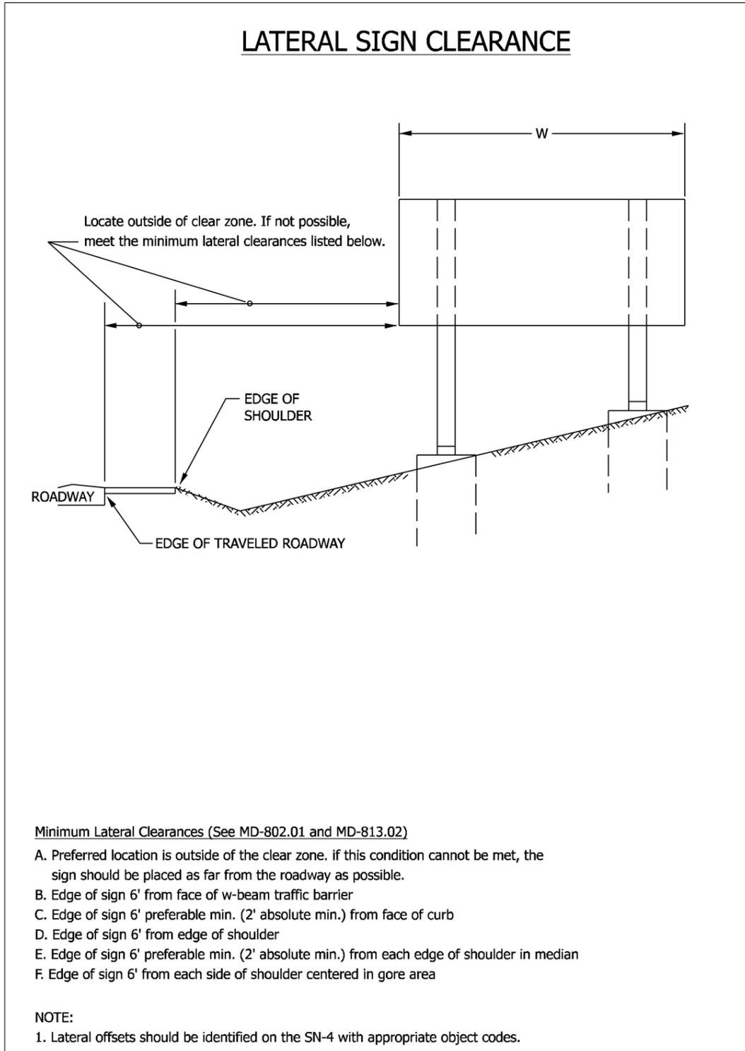
**Figure SN.42 - Lateral Sign Clearance**
