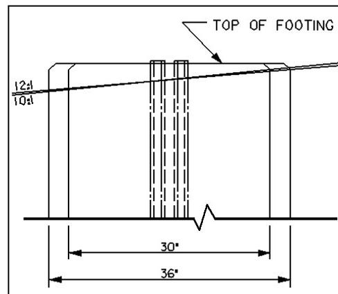
**Figure SN.34 - Slope Limits for Foundations**
