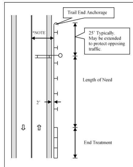
**Figure SN.36 - Typical Traffic Barrier Installation**
