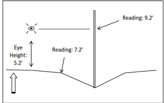
**Figure SN.4 - Roadside Elevation Readings**
