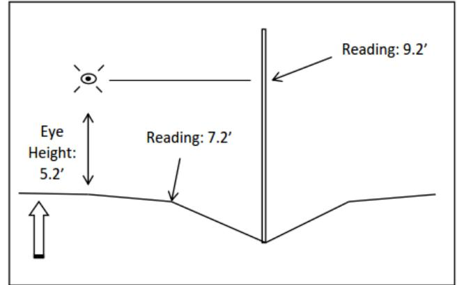
**Figure SN.4 - Roadside Elevation Readings**
