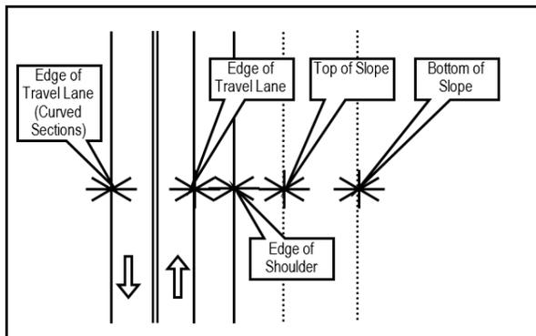
**Figure SN.3 - Typical Elevation Requirements**
