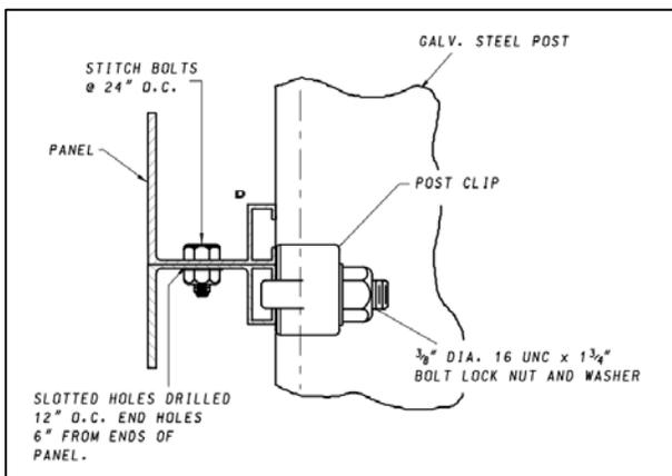
Figure SN.14 - Typical Extruded Panel
