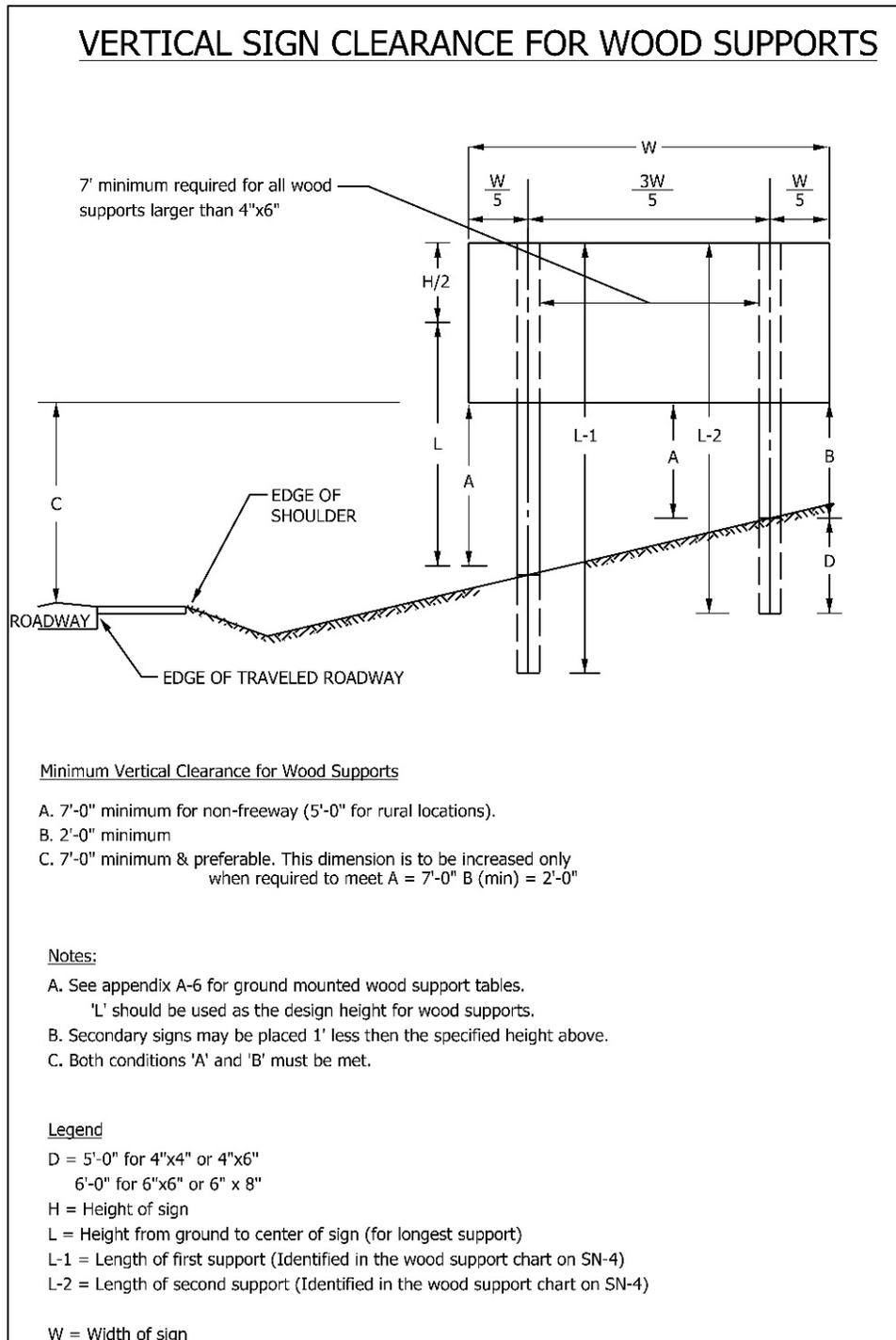
Figure SN.27 - Wood Support Vertical Clearance
