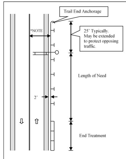
**Figure SN.36 - Typical Traffic Barrier Installation**
