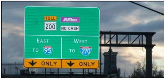
**Figure SN.10 - Negative Contrast "ONLY" Panels**
