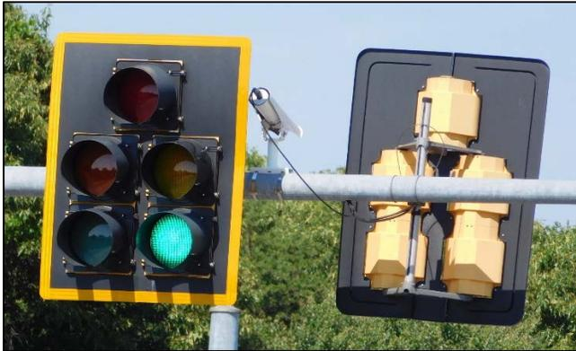
**Figure SG. 14 - Signal Backplates**
