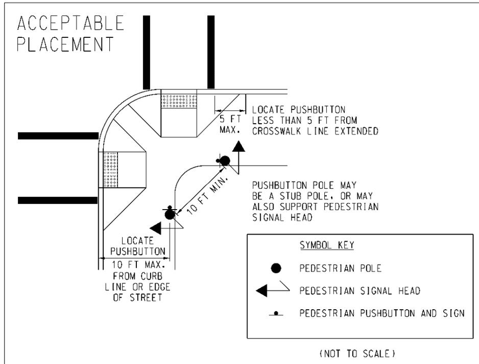
Figure SG. 31 - Acceptable Placement of APS
