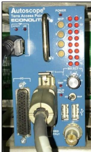
Figure SG. 20 - Video Interface Card (Close Up)
