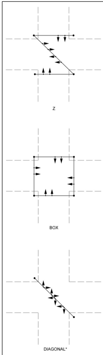
**Figure SG. 8 - Span Wire Signal Configurations**
