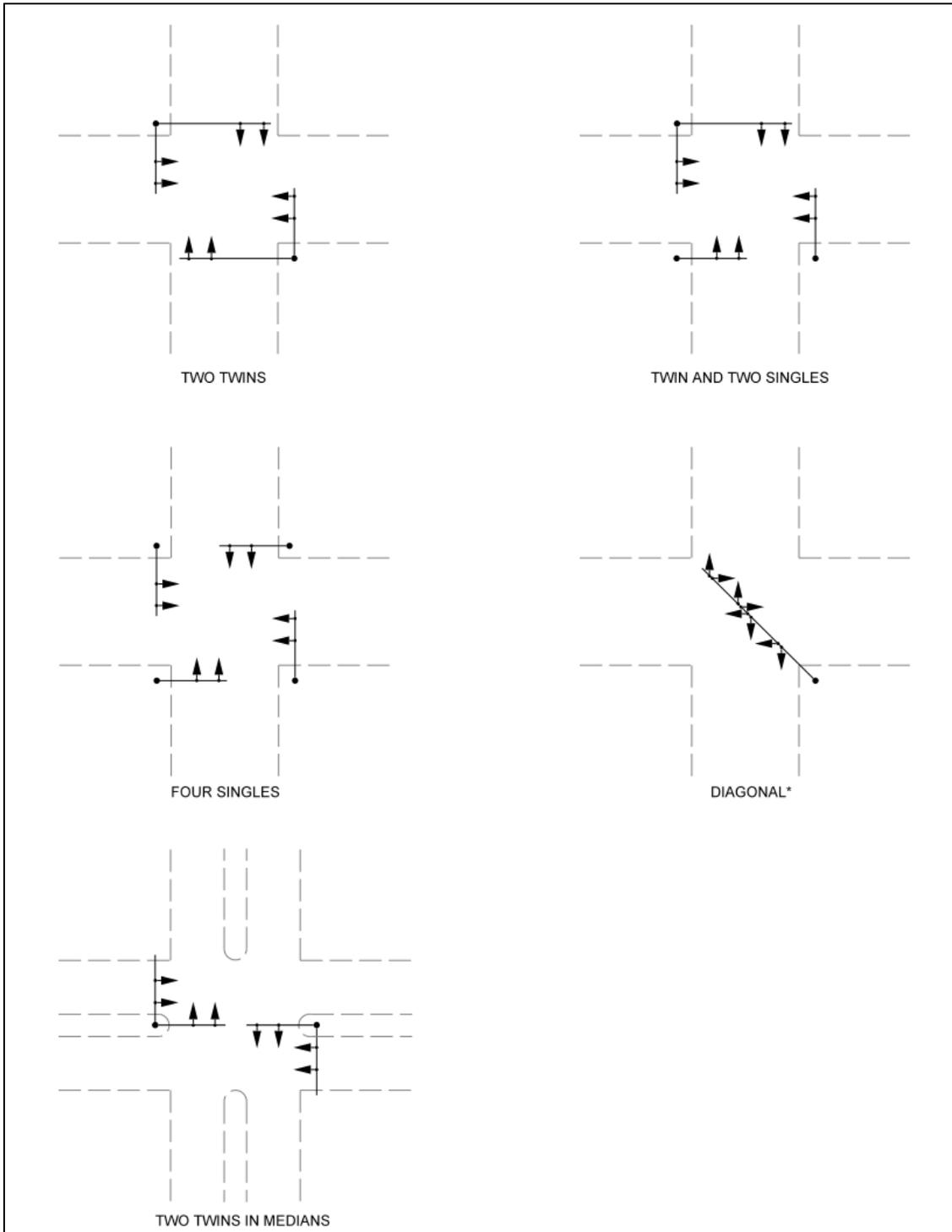
**Figure SG. 7 - Mast Arm Signal Configuration**
