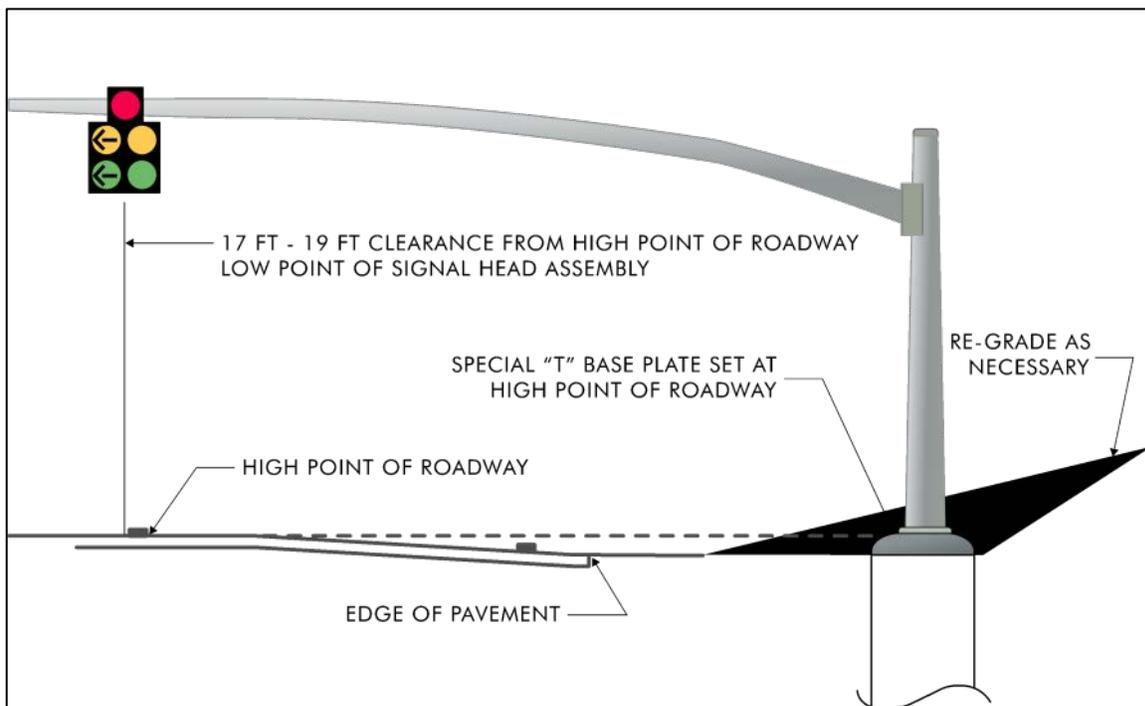
Figure SG. 6 - Special "T" Dimension Mast Arm Installation
