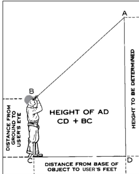
**Figure SG. 1 - Using a Teleheight; Source Hubbell Power Systems**
