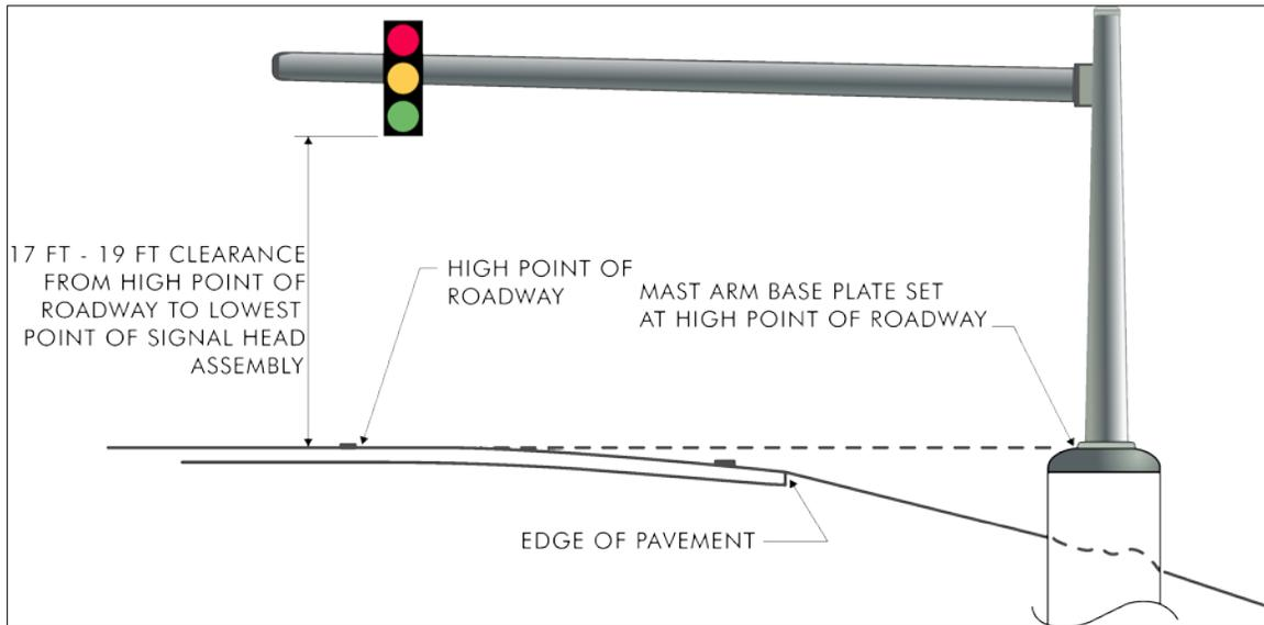
Figure SG. 5- Mast Arm Installation
