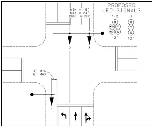
**Figure SG. 16 - Signal Head Horizontal Placement – Typical Signal Head Placements for Exclusive/Permissive Left Turn**
