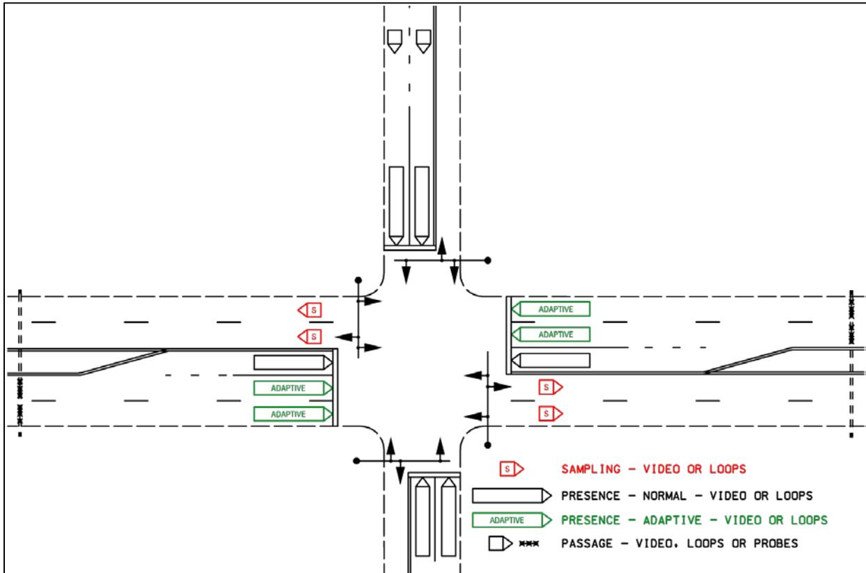
Figure SG. 26 - Detection Zone Types
