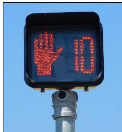
**Figure SG. 27 - Countdown Pedestrian Signal**
