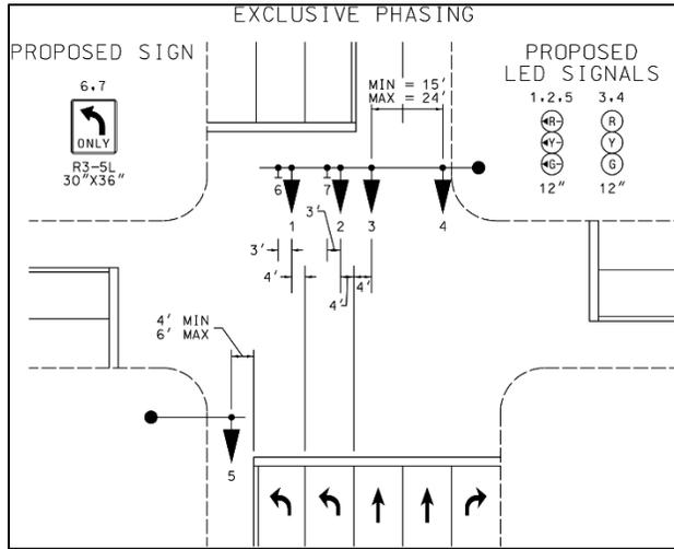
**Figure SG. 19 - Typical Signal Head Placements for Exclusive Double Left Turn**
