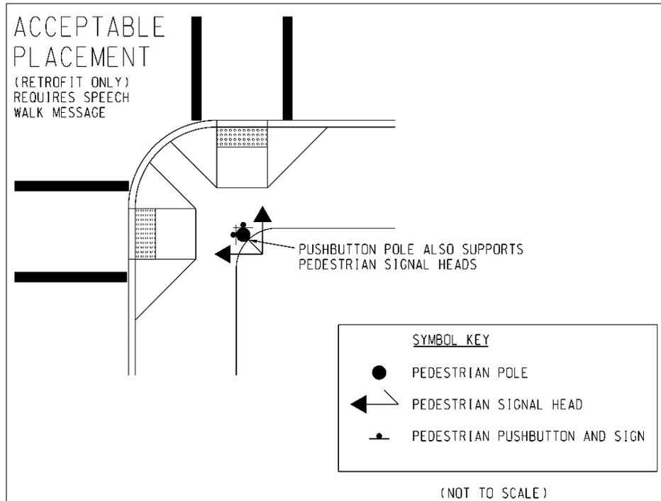
Figure SG. 33 - Retrofit Placement of APS
