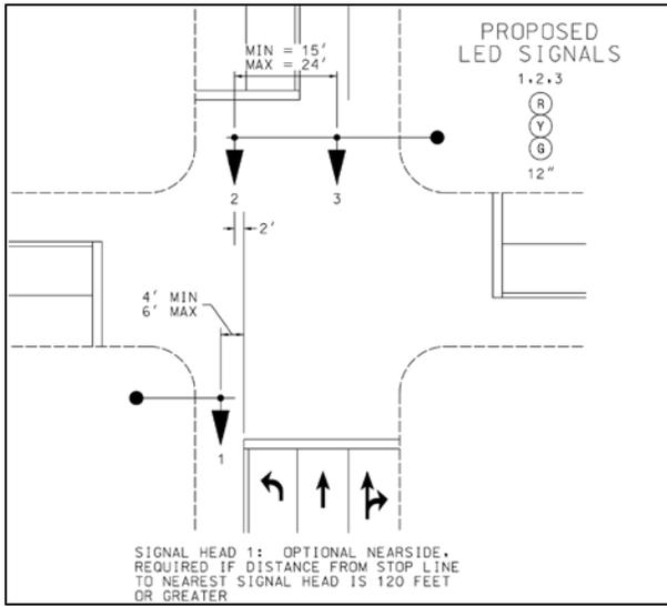
**Figure SG. 15 - Signal Head Horizontal Placement – Preferred for two far side and one near side three-section standard heads**
