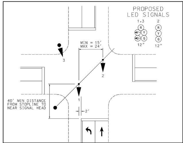
**Figure SG. 18 - Typical Far Left Turn Traffic Signal Head Location\***
