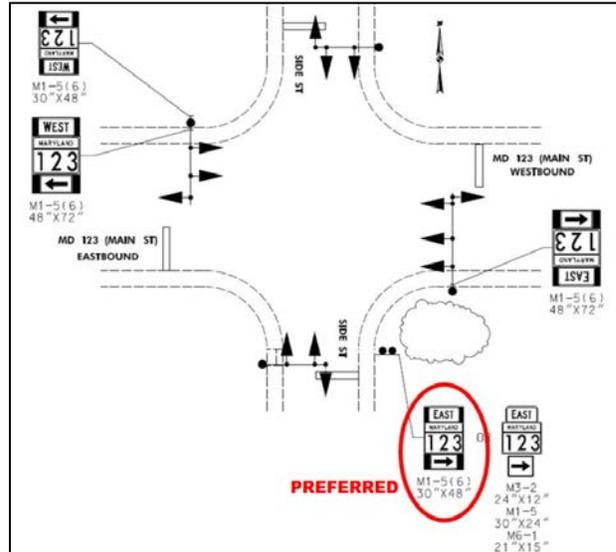
**Figure SG. 42 - Route Marker Assemblies at Signalized Intersections**
